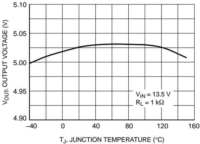
Figure 4. Output Voltage vs. Junction Temperature (5.0 V Version)
