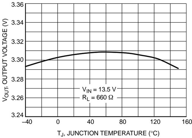
Figure 12. Output Voltage vs. Junction Temperature (3.3 V Version)
