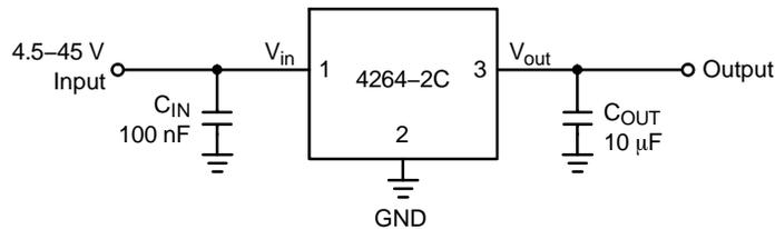
Figure 2. Applications Circuit
