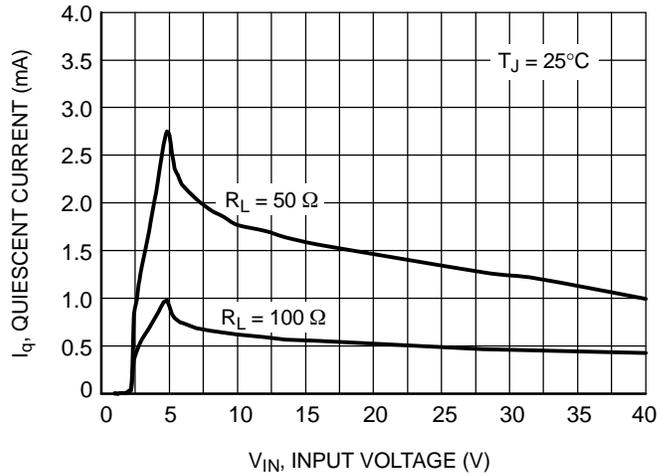
Figure 10. Quiescent Current vs. Input Voltage (5.0 V Version)
