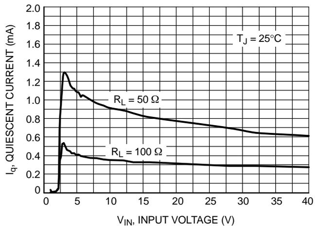
Figure 15. Quiescent Current vs. Input Voltage (3.3 V Version)
