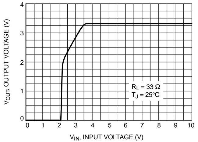
Figure 13. Output Voltage vs. Input Voltage (3.3 V Version)
