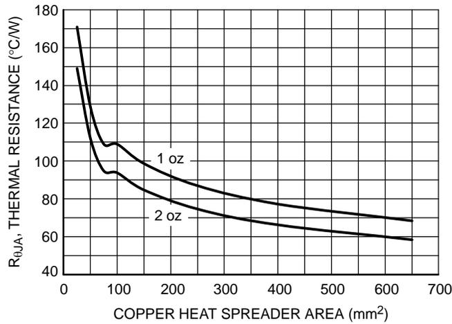
Figure 18. R<sub>θJA</sub> vs. Copper Spreader Area
