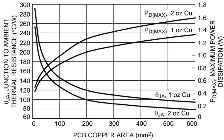
Figure 23.  $\theta_{JA}$  and  $P_{D(MAX)}$  vs. Copper Area
