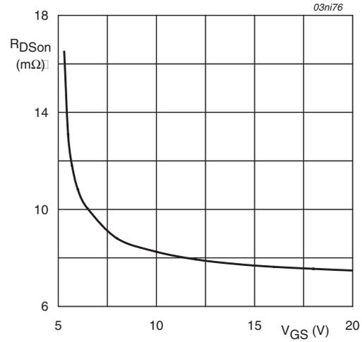
$$T_j = 25^\circ\text{C}; I_D = 50\text{A}$$
