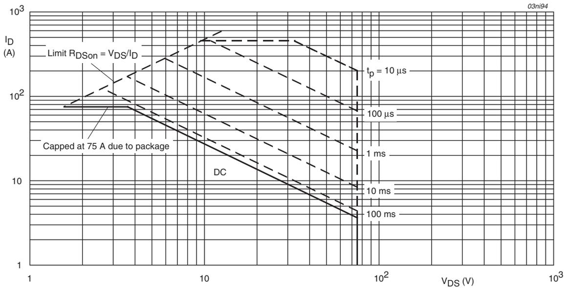
$T_{mb} = 25^\circ\text{C}; I_{DM}$  is single pulse
