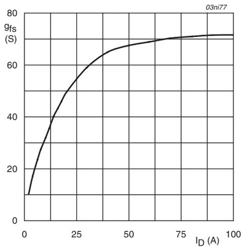
$T_j = 25^\circ\text{C}; V_{DS} = 25\text{V}$
