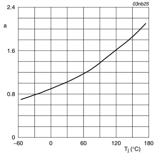
$$a = \frac{R_{DSon}}{R_{DSon(25^\circ\text{C})}}$$
