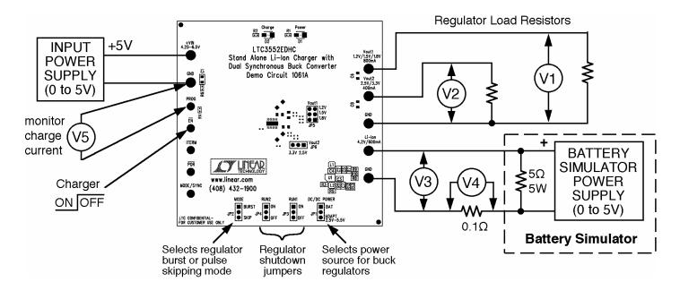
Figure 1. Demonstration Circuit Test Setup
