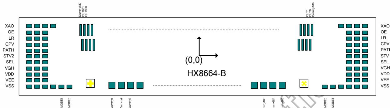
Chip size: 20212  $\mu\text{m}$  x 674 $\mu\text{m}$  (scribe line included)
