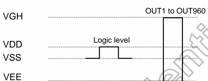
The logic levels of CPV, L/R, OE, /XAO, MODE0, MODE1, SEL, STV1 and STV2 have to swing between VDD for "H" and VSS for "L".
