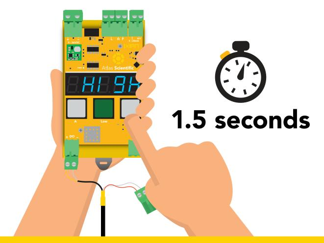
You may see the readings start to rise slowly after calibration. This is not uncommon. Simply press "**high**" calibration button again. This can be done many times; each time, your calibration will become more accurate. "*Prefect Calibration*" does not exist. It's is a psychological trap. Limit high point calibration attempts to no more than 10 minutes.
