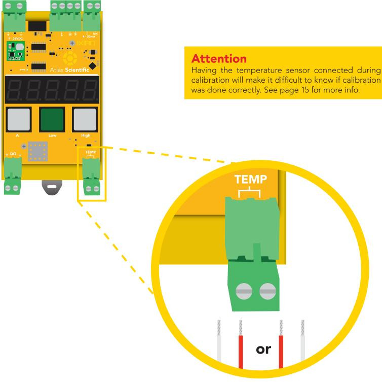
Either method of wiring will produce the same result. *There is no polarity.*
