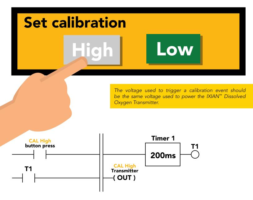
A calibration event will only trigger if the corresponding input pin has been held high for 200ms. Holding the line for more then 200ms will have no effect.
