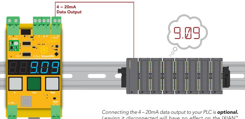
Leaving it disconnected will have no effect on the IXIAN™ Dissolved Oxygen Transmitter's operation.
