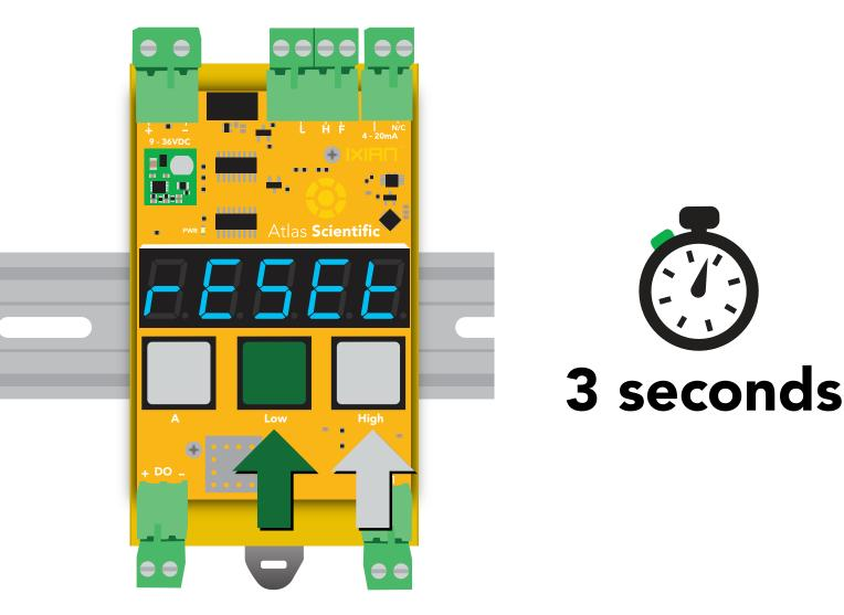
Press and hold the **Low** and **High** buttons again to confirm the factory reset. To cancel a factory reset, press the **A** button
