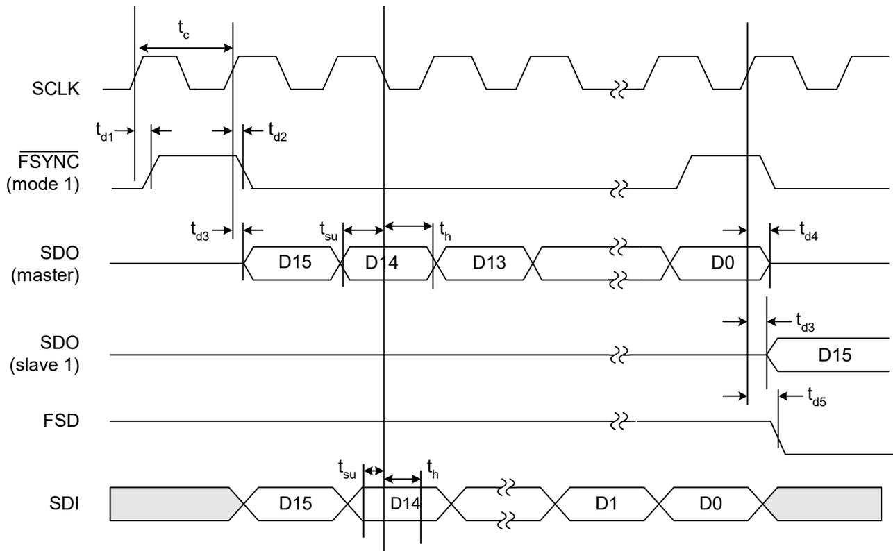
**Figure 5. Serial Interface Timing Diagram (DCE = 1, FSD = 1)**
