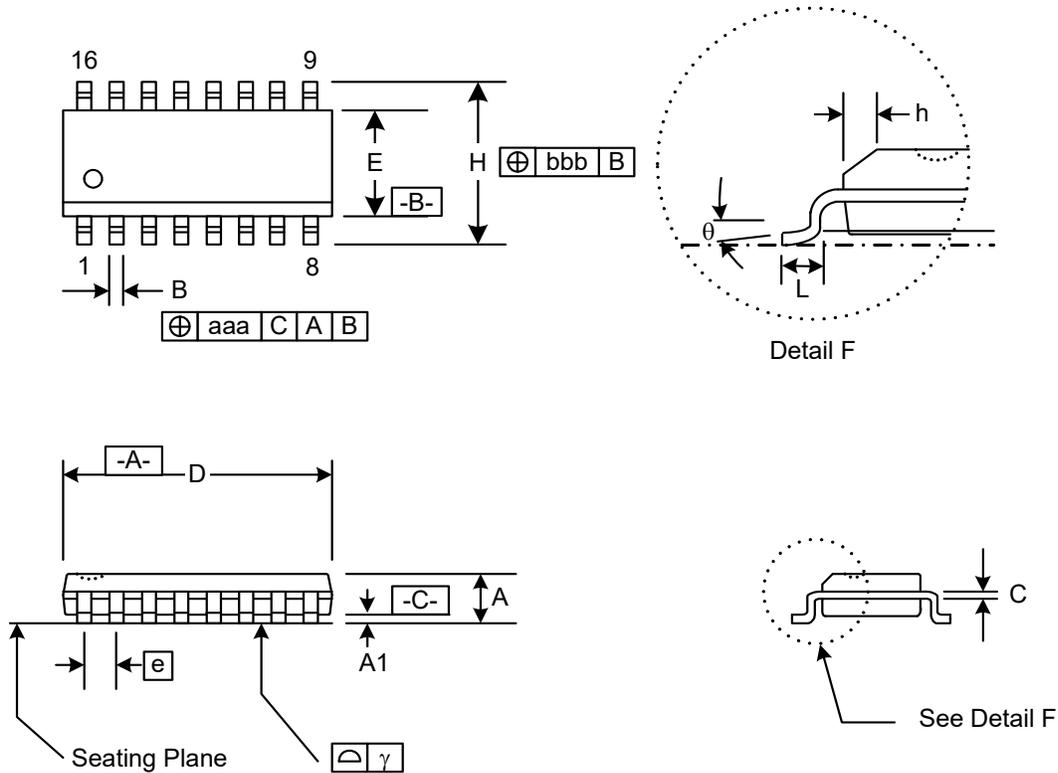
Figure 37. 16-pin Small Outline Integrated Circuit (SOIC) Package
