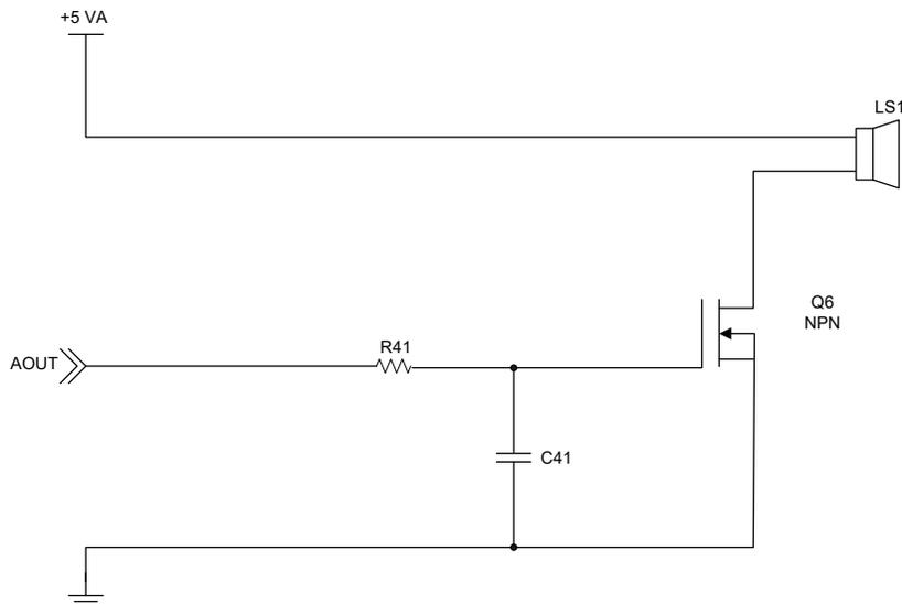
**Figure 18. AOUT PWM Circuit for Call Progress**
