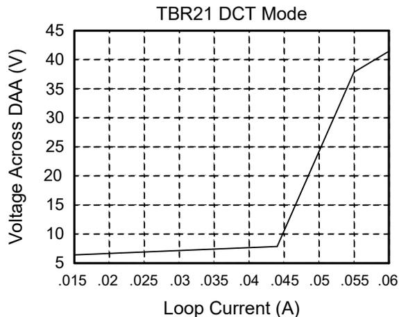
**Figure 21. TBR21 Mode I/V Characteristics, DCV[1:0] = 11, MINI[1:0] = 00, ILIM = 1**
