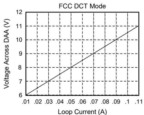
**Figure 20. FCC Mode I/V Characteristics, DCV[1:0] = 11, MINI[1:0] = 00, ILIM = 0**
