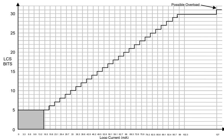
**Figure 19. Typical Loop Current LCS Transfer Function**
