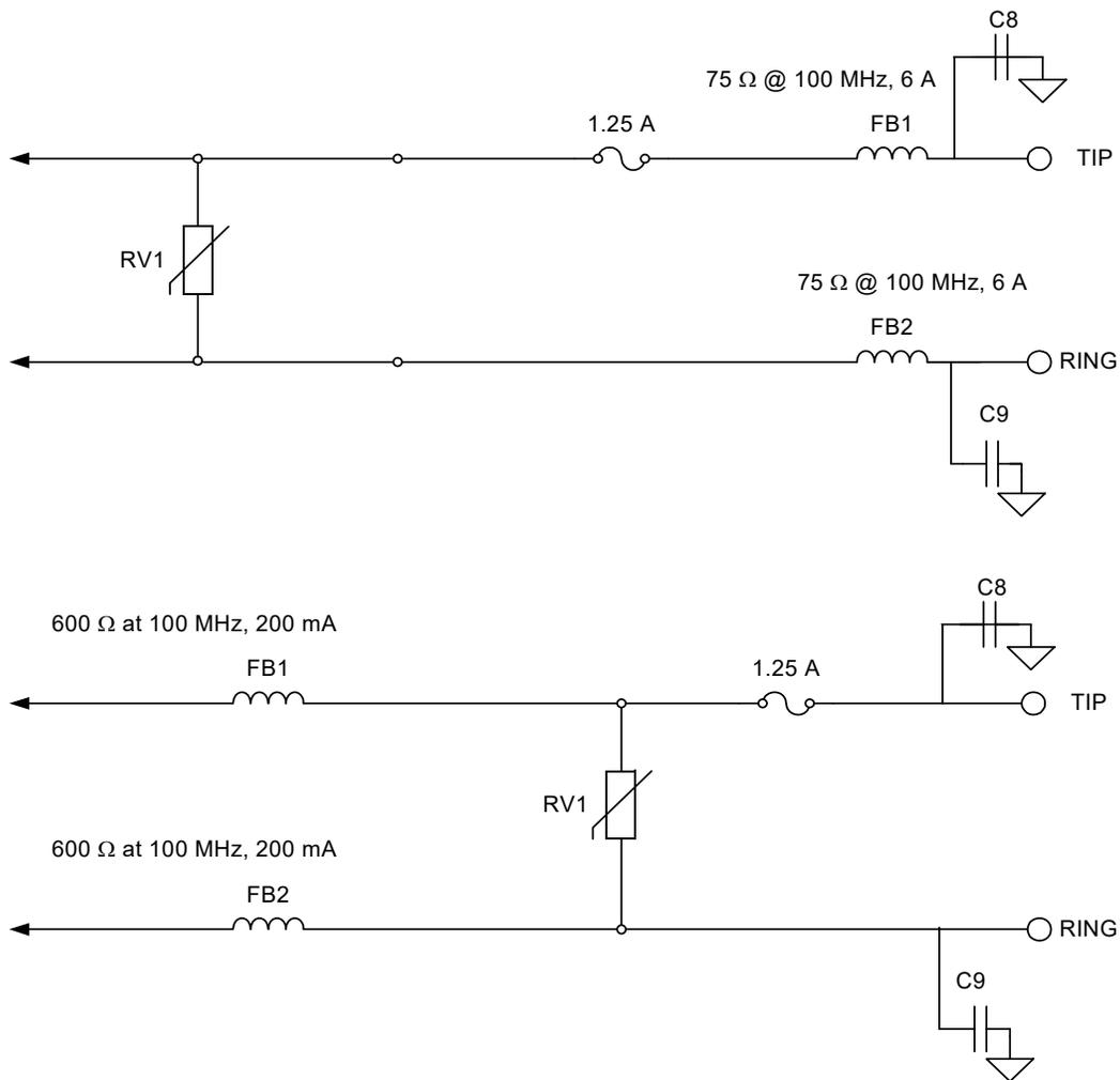
**Figure 38. Circuits that Pass all UL1950 Overvoltage Tests**
