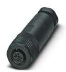
Bus system connector, 5-position, Socket straight M12, B-coded, Screw connection, knurl material: Plastic, cable gland Pg9, external cable diameter 6 mm ... 8 mm
