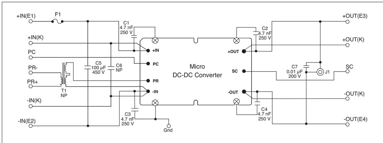
Figure 5: Micro DC-DC converter Evaluation Board schematic
