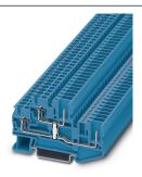
Double-level terminal block, With equipotential bonder, nom. voltage: 500 V, nominal current: 22 A, connection method: Spring-cage/plug-in connection, 1st and 2nd level connection left, Rated cross section: 2.5 mm², cross section: 0.08 mm² - 4 mm², 1st and 2nd level connection right, mounting type: NS 35/15, NS 35/7,5, color: blue
