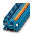
Feed-through terminal block, Connection type: Quick connection, Spring-cage connection, Cross section: 0.25 mm² - 1.5 mm², AWG :24- 16, Width: 5.2 mm, Color: blue, Mounting: NS 35/7,5, NS 35/15
