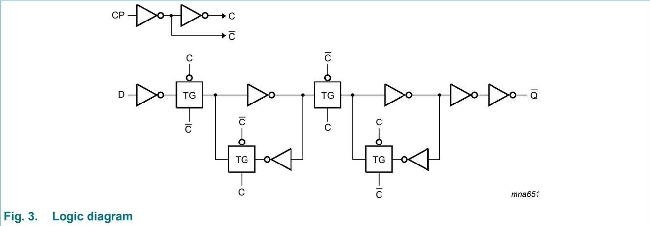
Fig. 3. Logic diagram
