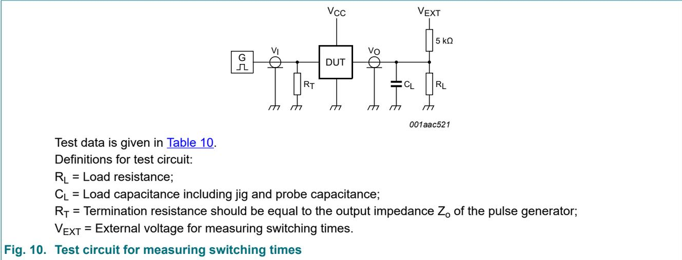
**Fig. 10. Test circuit for measuring switching times**
