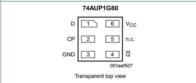
Fig. 6. Pin configuration SOT1115 and SOT1202 (XSON6)
