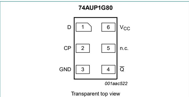
Fig. 5. Pin configuration SOT886 (XSON6)
