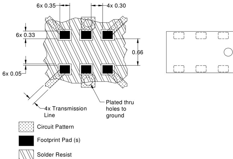
Dimensions are in Millimeters
