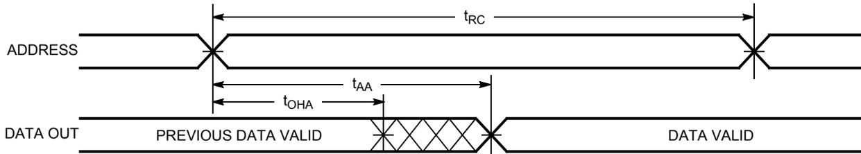
Figure 4. Read Cycle No. 2 ( $\overline{OE}$  Controlled) [12, 13]
