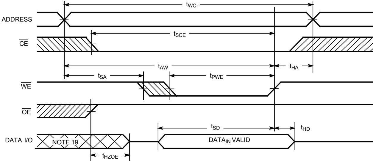
Figure 7. Write Cycle No. 3 ( $\overline{WE}$  Controlled,  $\overline{OE}$  LOW) [17, 18]
