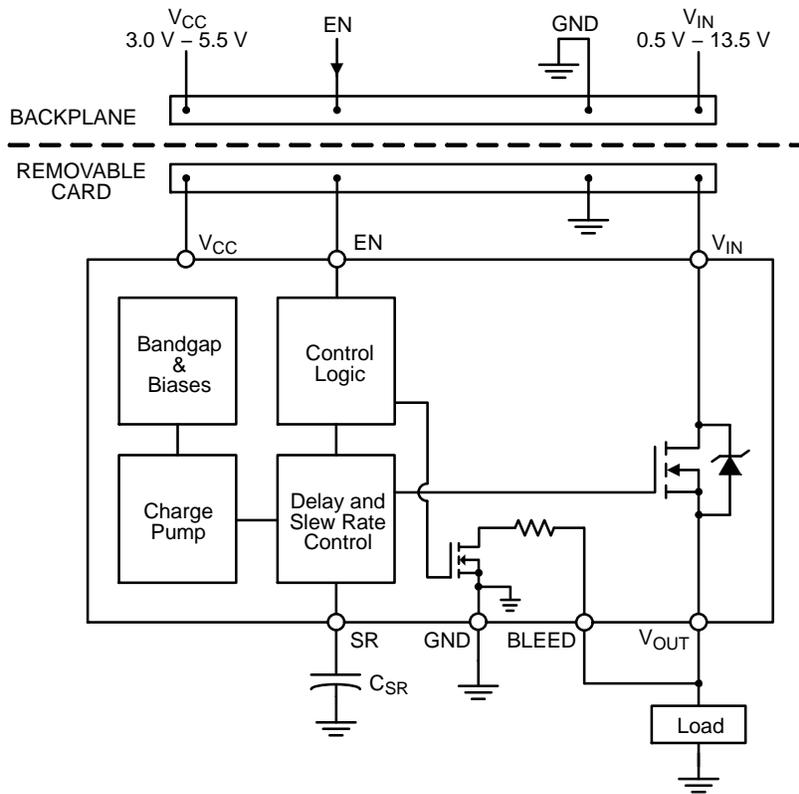
**Figure 32. NCP45525 Typical Application Diagram – Hot Swap**
