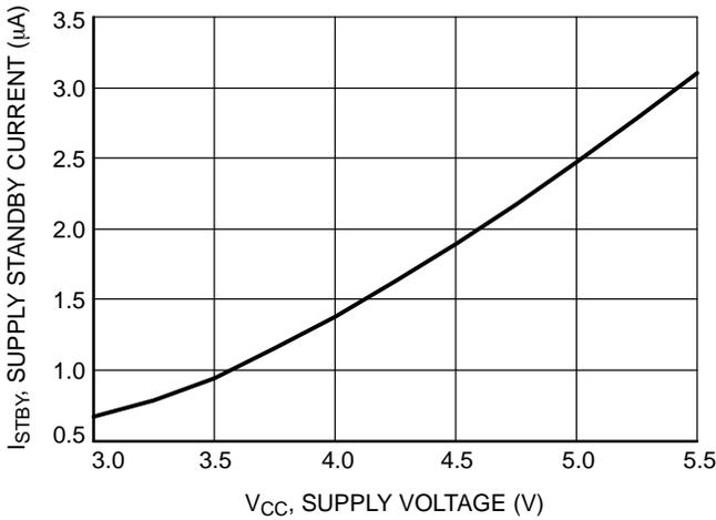
Figure 5. Supply Standby Current vs. Supply Voltage
