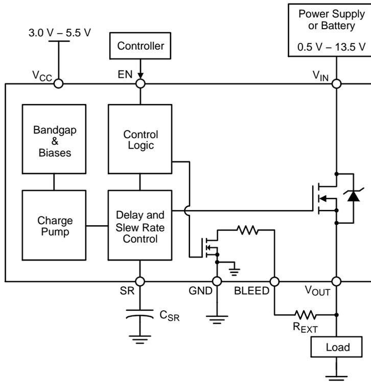
**Figure 31. NCP45525 Typical Application Diagram – Load Switch**
