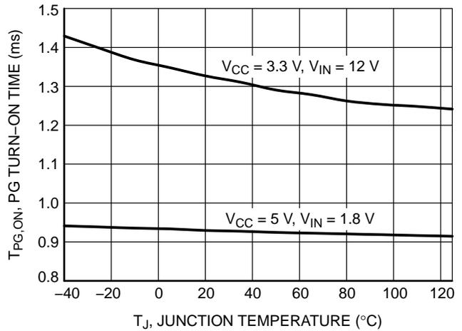
**Figure 24. Power Good Turn-on Time vs. Temperature**
