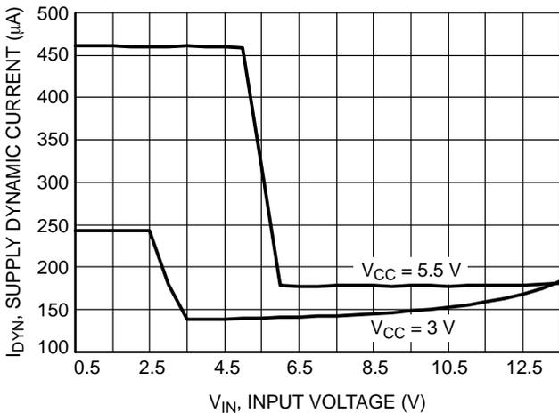
Figure 7. Supply Dynamic Current vs. Input Voltage
