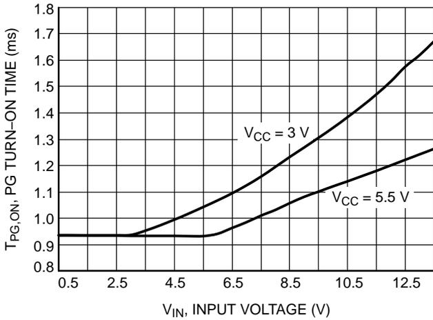
**Figure 23. Power Good Turn-on Time vs. Input Voltage**
