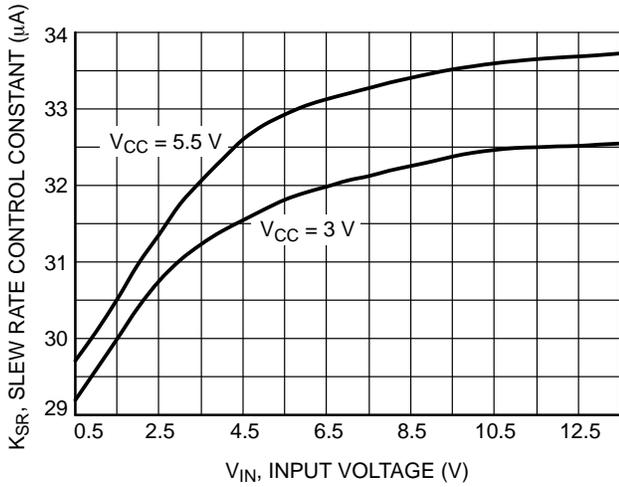
**Figure 15. Slew Rate Control Constant vs. Input Voltage**
