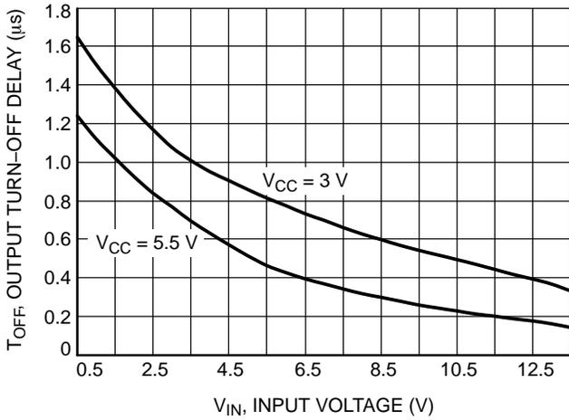
**Figure 21. Output Turn-off Delay vs. Input Voltage**
