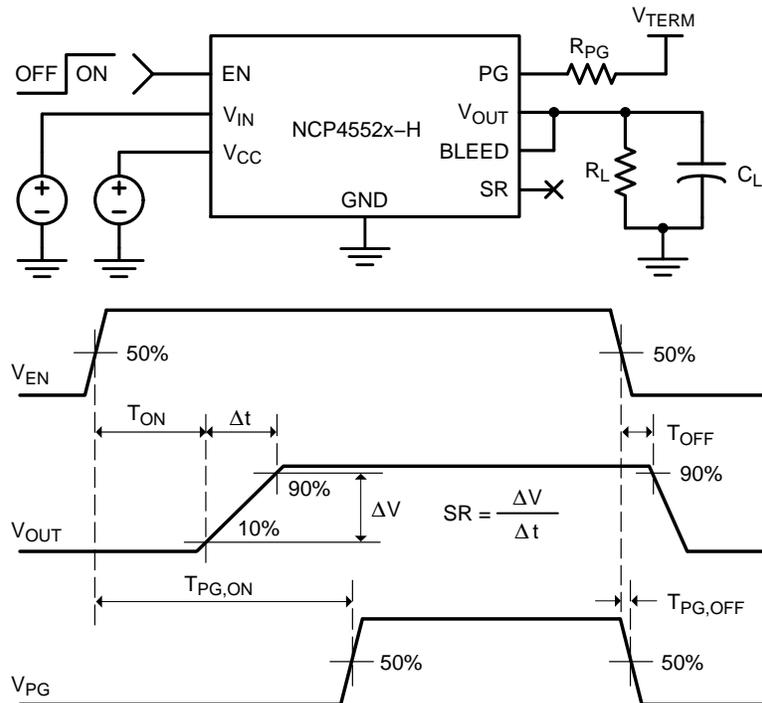
**Figure 2. Switching Characteristics Test Circuit and Timing Diagram**
