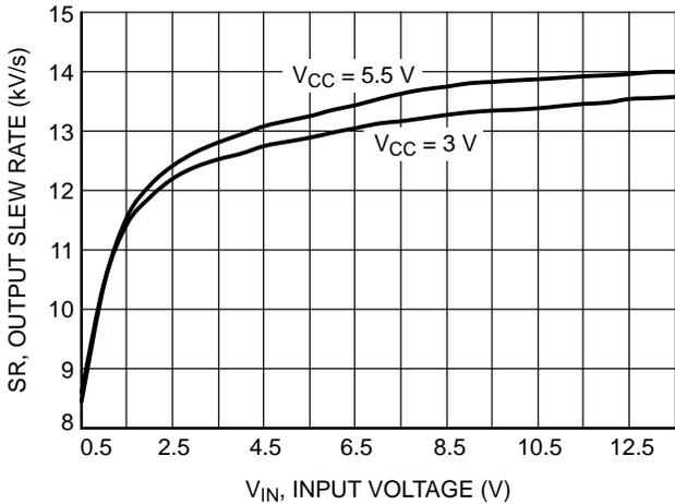
**Figure 17. Output Slew Rate vs. Input Voltage**
