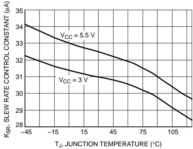
**Figure 16. Slew Rate Control Constant vs. Temperature**
