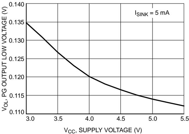
**Figure 13. PG Output Low Voltage vs. Supply Voltage**
