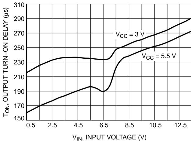
**Figure 19. Output Turn-on Delay vs. Input Voltage**
