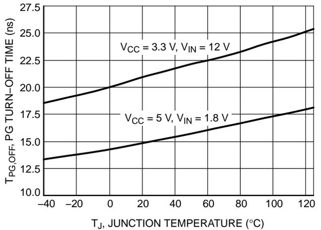
**Figure 26. Power Good Turn-off Time vs. Temperature**
