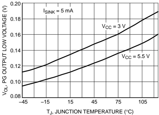
**Figure 14. PG Output Low Voltage vs. Temperature**
