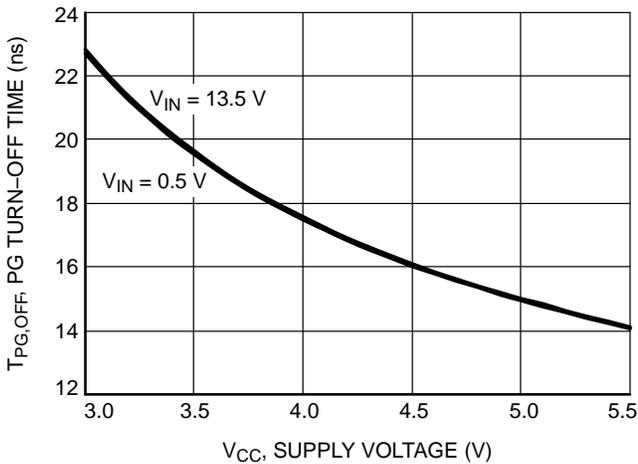
**Figure 25. Power Good Turn-off Time vs. Supply Voltage**
