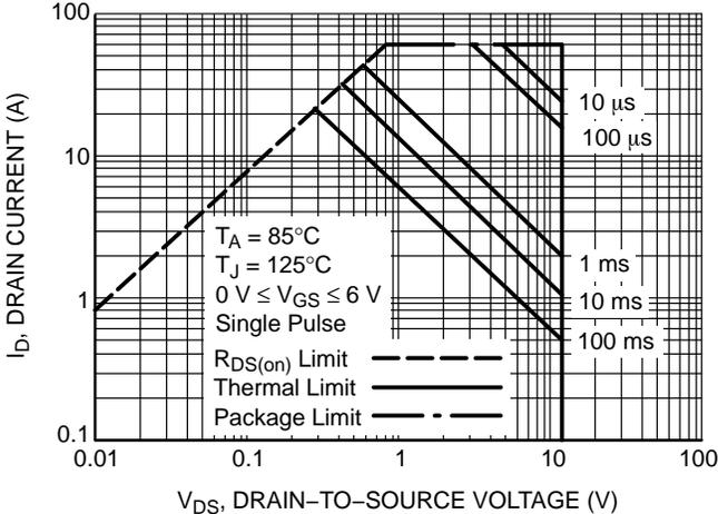
**Figure 27. Maximum Rated Forward Biased Safe Operating Area**
