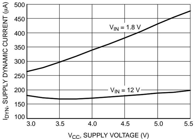
Figure 8. Supply Dynamic Current vs. Supply Voltage
