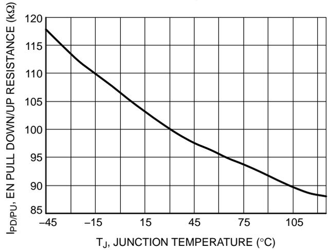
**Figure 12. EN Pull Down/Up Resistance vs. Temperature**
