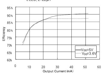
3. Efficiency VS Input Voltage I<sub>LED</sub>=20mA, 10 LED
