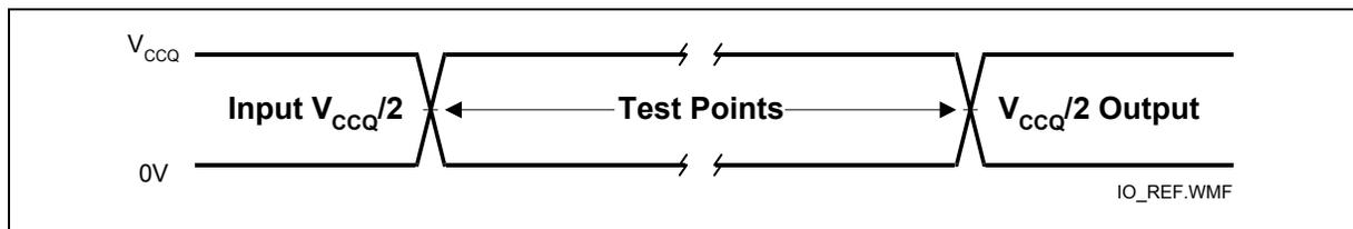
**Note:** AC test inputs are driven at  $V_{CCQ}$  for Logic "1" and  $0V$  for Logic "0." Input/output timing begins/ends at  $V_{CCQ}/2$ . Input rise and fall times (10% to 90%) < 5 ns. Worst-case speed occurs at  $V_{CC} = V_{CCMin}$ .
