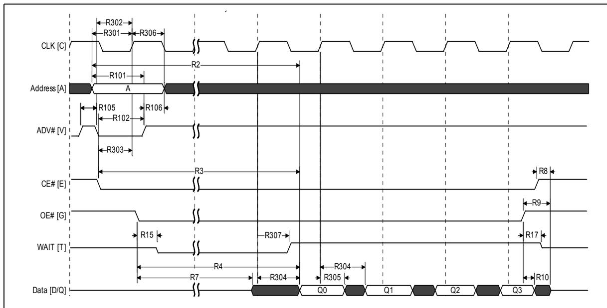
**Note:** WAIT is driven per OE# assertion during synchronous array or non-array read. WAIT asserted during initial latency and deasserted during valid data (RCR.10=0, WAIT asserted low).
