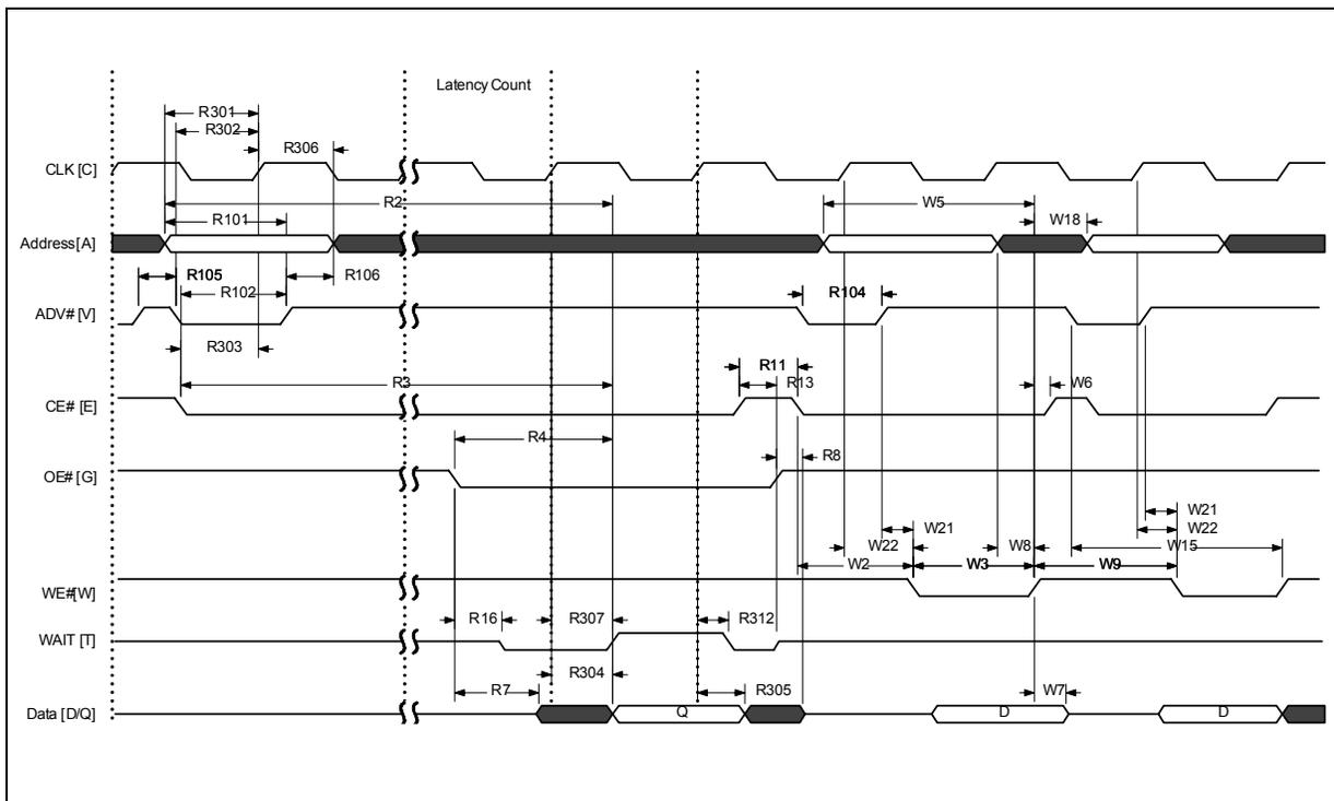
**Note:** WAIT shown deasserted and High-Z per OE# deassertion during write operation (RCR 10=0, WAIT asserted low). Clock is ignored during write operation.
