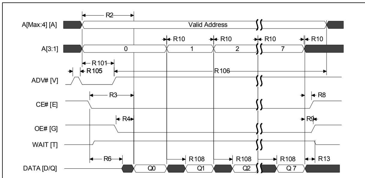
**Note:** WAIT shown deasserted during asynchronous read mode (RCR.10=0, WAIT asserted low).
