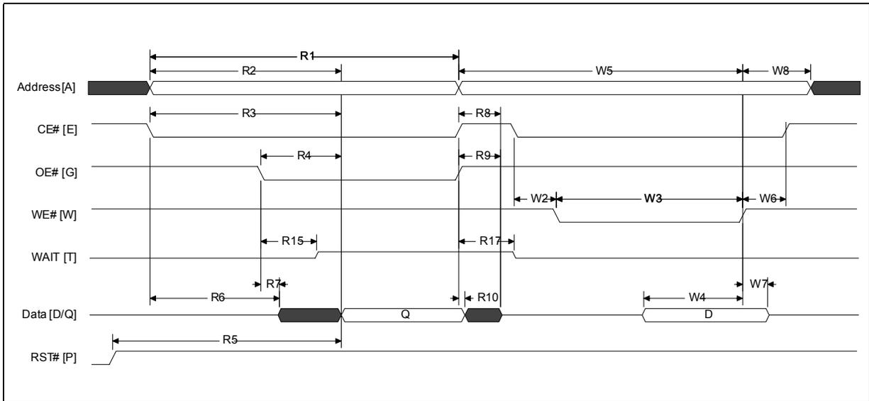
**Note:** WAIT deasserted during asynchronous read and during write. WAIT High-Z during write per OE# deasserted.
