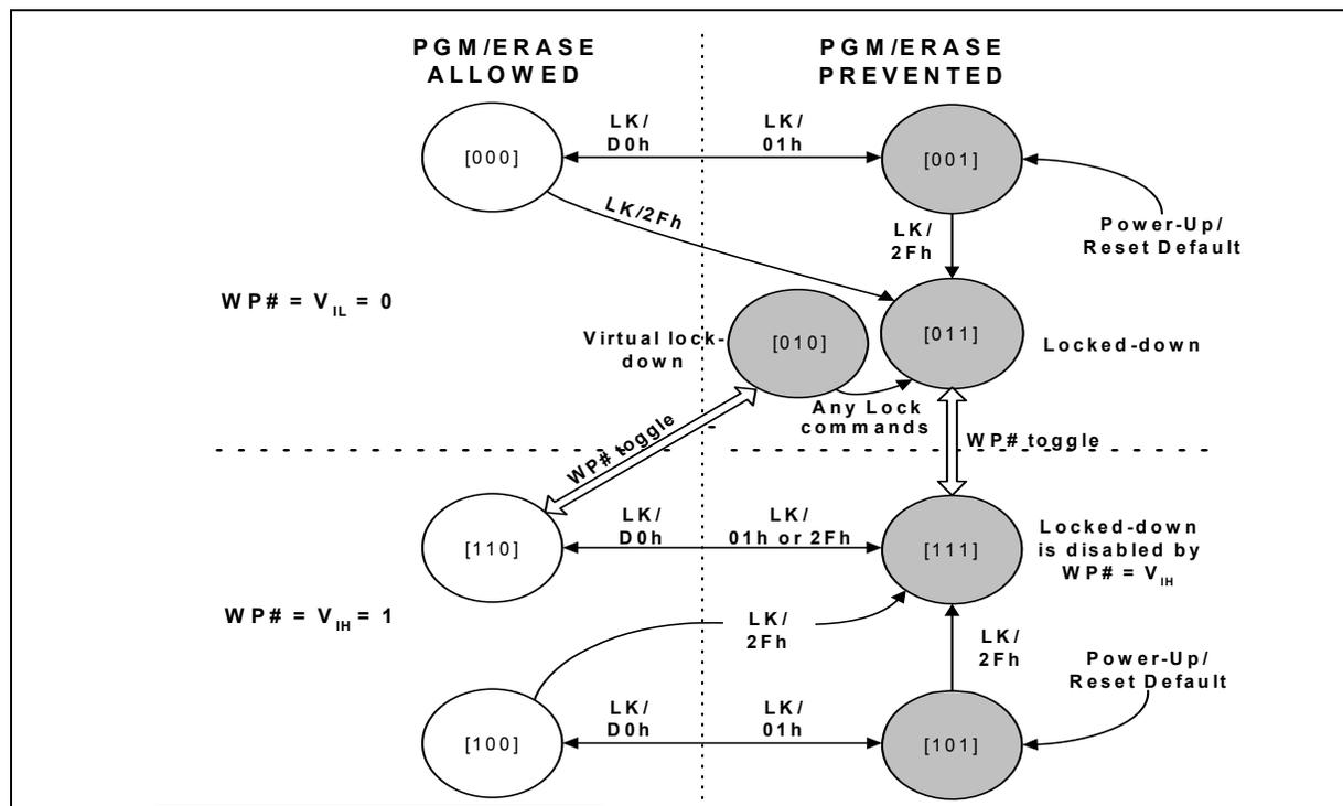
**Note:** LK: Lock Setup Command, 60h; LK/D0h: Unlock Command; LK/01h: Lock Command; LK/2Fh: Lock-Down Command.
