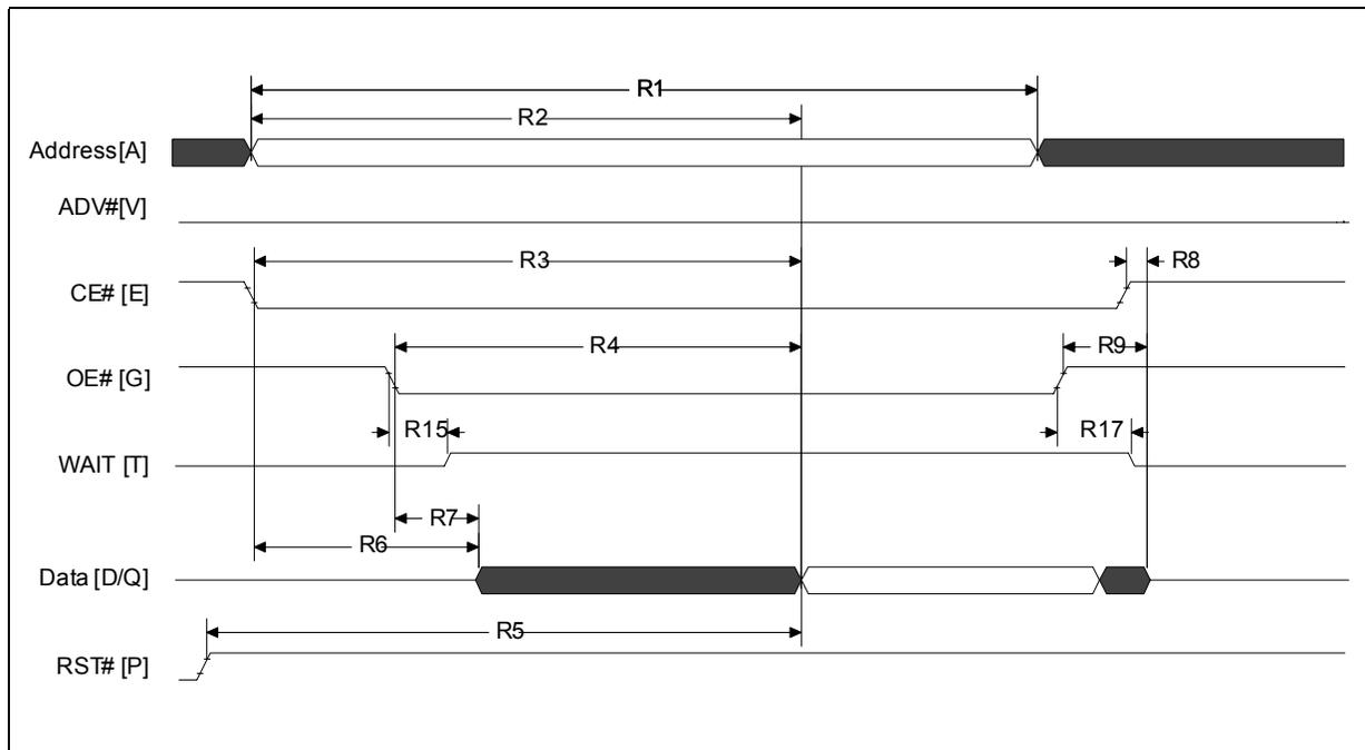
**Note:** WAIT shown deasserted during asynchronous read mode (RCR.10=0, WAIT asserted low).
