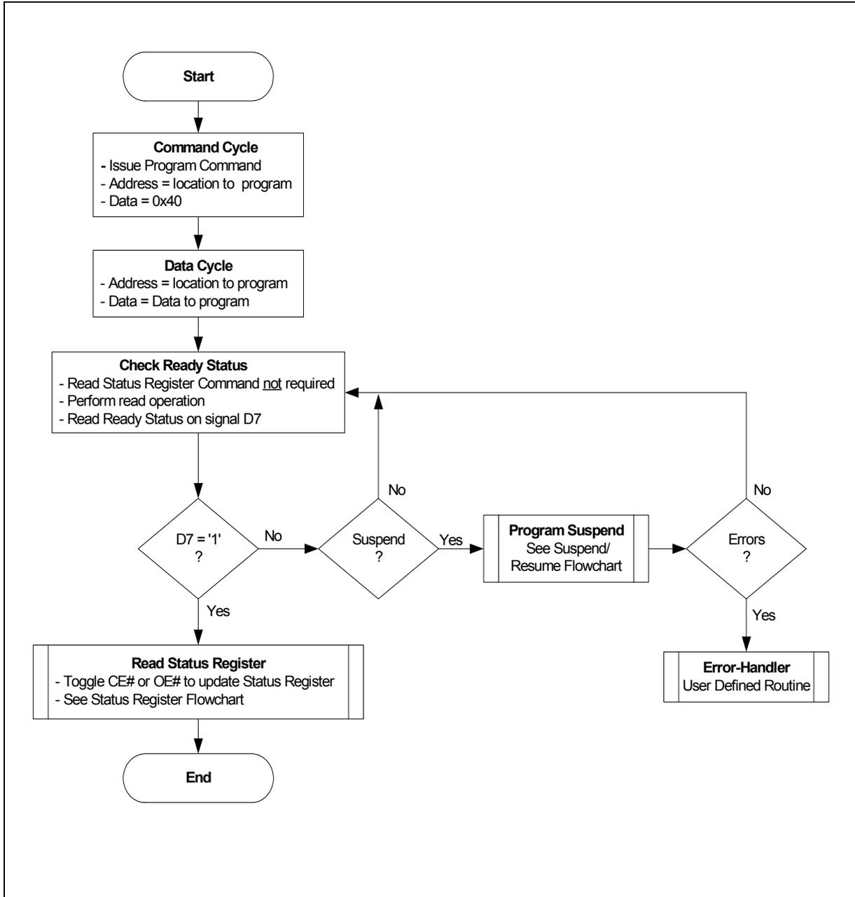
Figure 30: Program Suspend/Resume Flowchart
