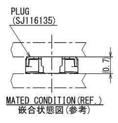
Note 1) Dimension  $3\pm0.05$  is recommended in case repair is needed.
