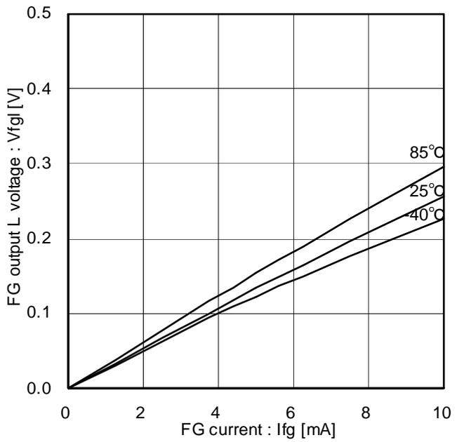
Figure 14. FG output L voltage (Temperature characteristics)
