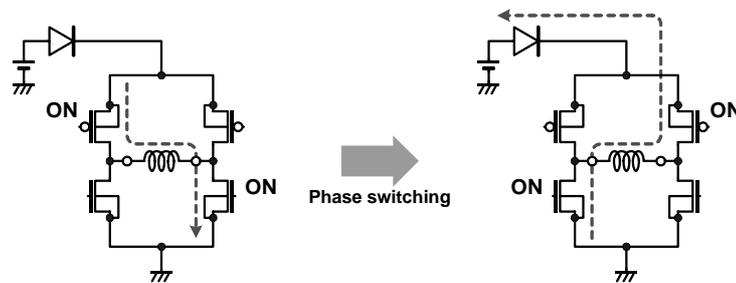
Figure 27. Vcc voltage rise by back electromotive force
