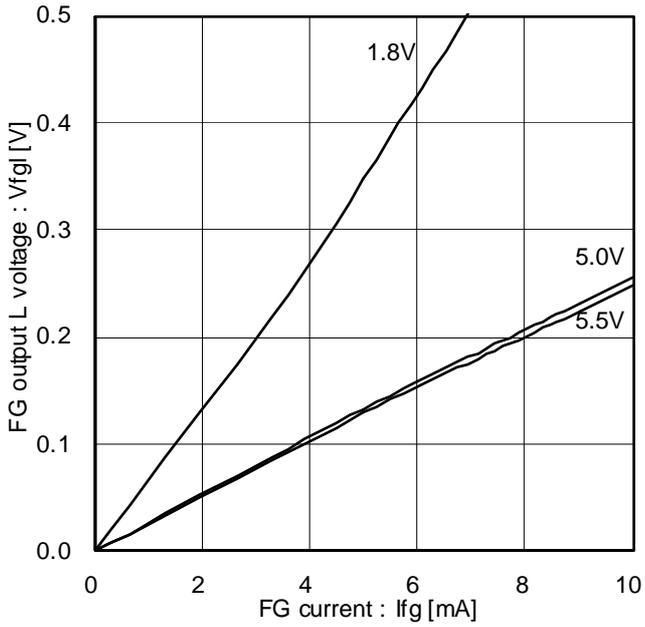
Figure 15. FG output L voltage (Voltage characteristics)
