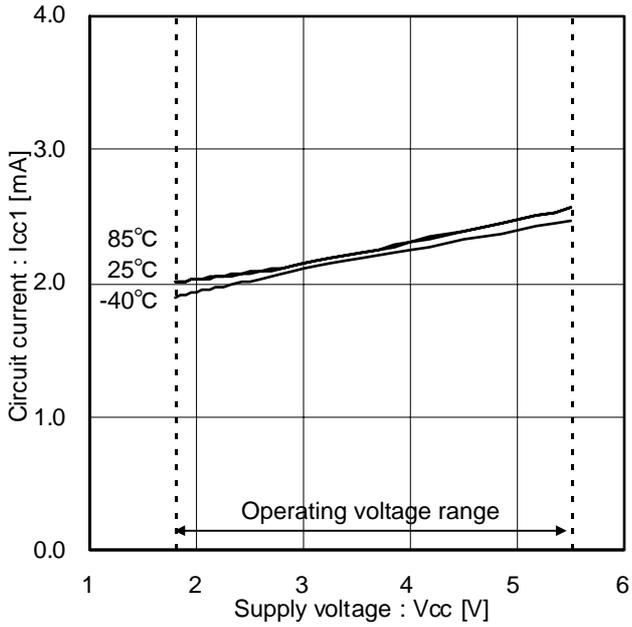
Figure 3. Circuit current 1
