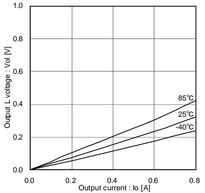
Figure 10. Output L voltage (Temperature characteristics)
