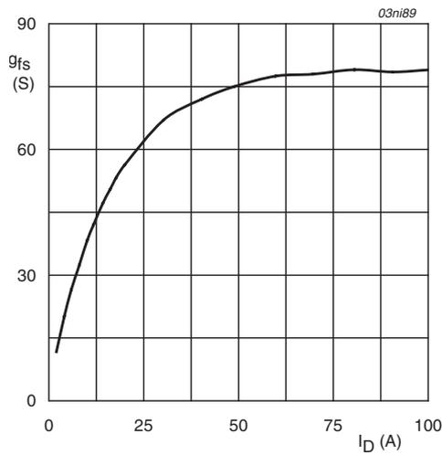
$T_j = 25\text{ °C}; V_{DS} = 25\text{ V}$
