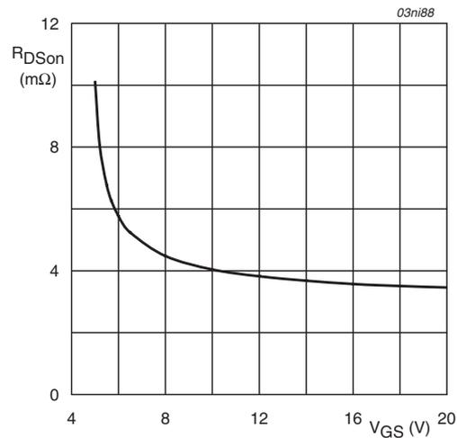
$T_j = 25\text{ }^\circ\text{C}$ ;  $I_D = 50\text{ A}$
