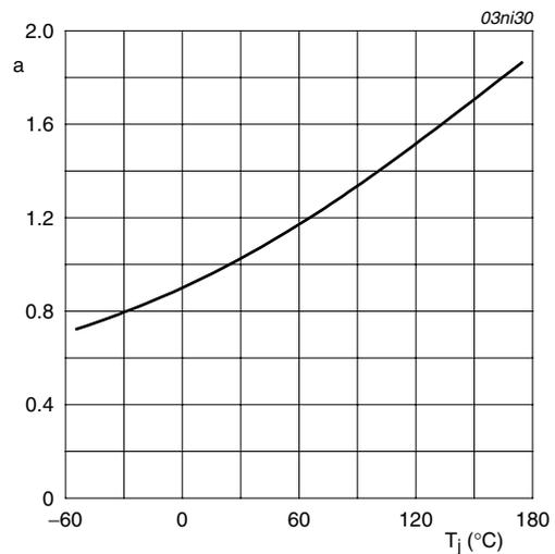
$$a = \frac{R_{DSon}}{R_{DSon(25^\circ\text{C})}}$$
