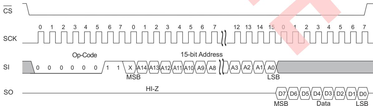
**Figure 13. Burst Mode Read Instruction Timing**
