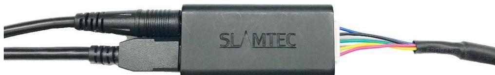
*Figure 2-2 Connect the USB Adapter to PC via Micro-USB Cable*
