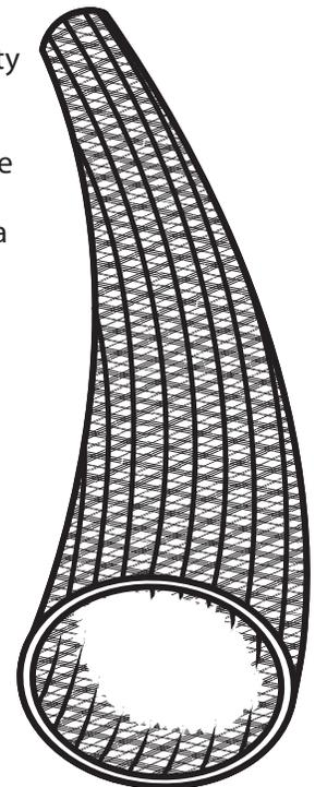
■ F360° braid is lightweight and quiet. It will bend to a tight radius without distorting, and it will not impair or affect the flexibility of harnesses.
