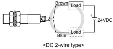
When using DC 2-wire type proximity sensor, the load must be connected, otherwise internal components may be damaged. The load can be connected to either wire.
