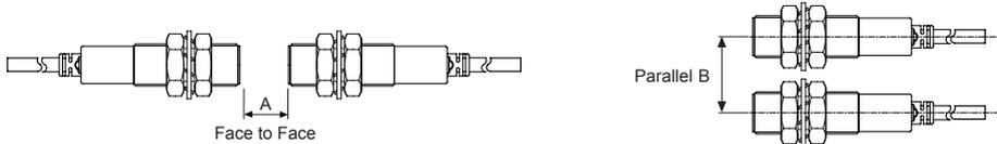
When sensors are mounted on metallic panel, it is required to protect the sensors from being affected by any metallic object except target. Therefore, be sure to provide a minimum distance as below chart indicates.
