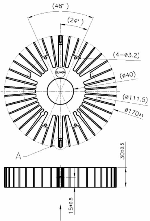
Assembly direction of customer's LED Module
