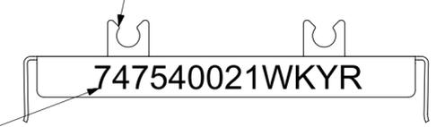
P/N AND WEEK/YEAR DATE CODE TO BE PRINTED ON BACK OF COMPLETED CAGE ASSEMBLY APPROXIMATELY AS SHOWN.
