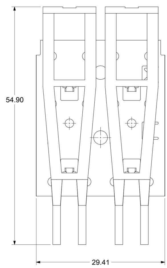
LIGHT PIPES SECURED TO METAL CAGE COVER
