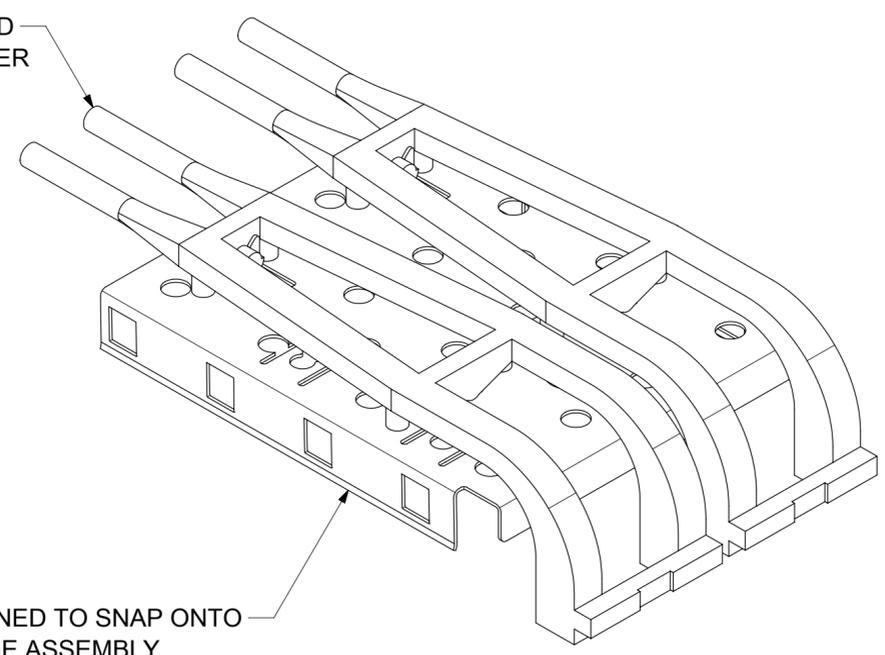
COVER DESIGNED TO SNAP ONTO THE SFP+ CAGE ASSEMBLY
