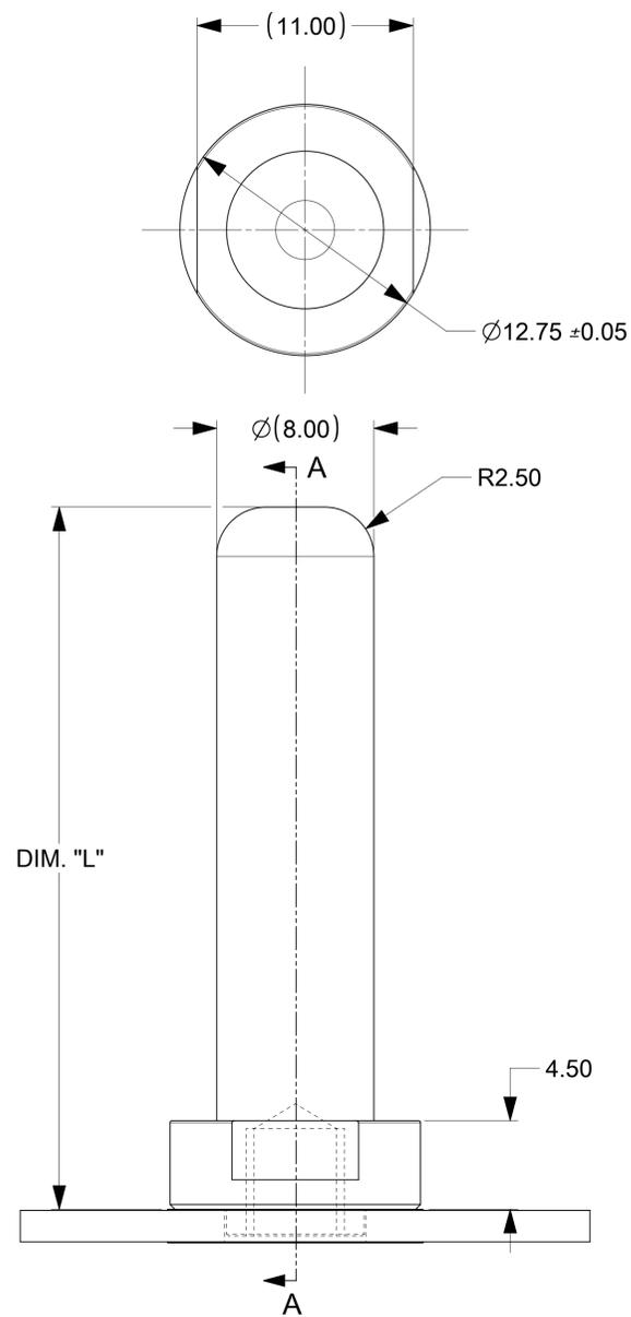
MINIMUM BOARD THICKNESS IS 1.58MM
