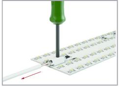
Inserting/removing fine-stranded conductors by lightly pressing on a push-button.
