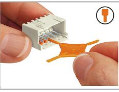
Coding a male header (via coding key carrier and two keys for male header, see symbol).
