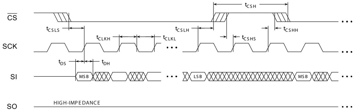
**Figure 14-2.** Serial Output Timing
