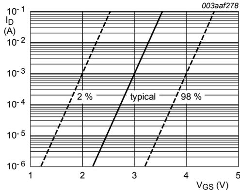
$T_j = 25\text{ }^\circ\text{C}; V_{DS} = V_{GS}$
