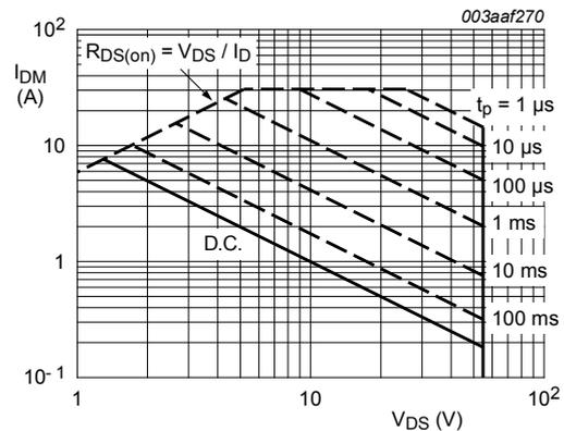
$T_{sp} = 25\text{ }^{\circ}\text{C}$ ;  $I_{DM}$  is single pulse
