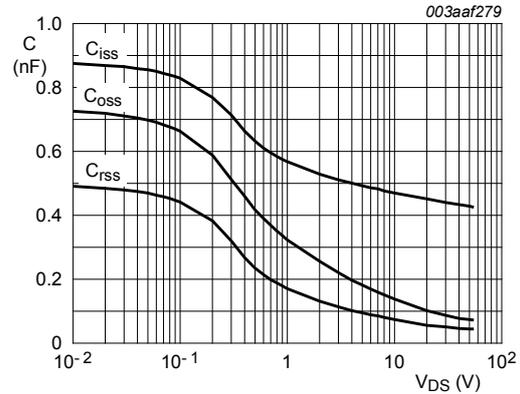
$V_{GS} = 0\text{ V}; f = 1\text{ MHz}$
