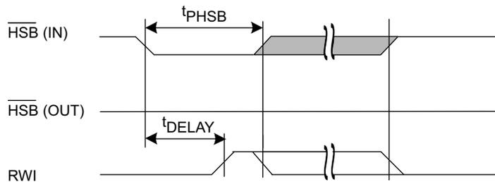
$\overline{HSB}$  pin is driven HIGH to  $V_{CC}$  only by Internal 100 K $\Omega$  resistor, HSB driver is disabled SRAM is disabled as long as  $\overline{HSB}$  (IN) is driven LOW.
