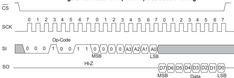
**Figure 17. Fast RTC Read (FAST\_RDRTC) Instruction Timing**
