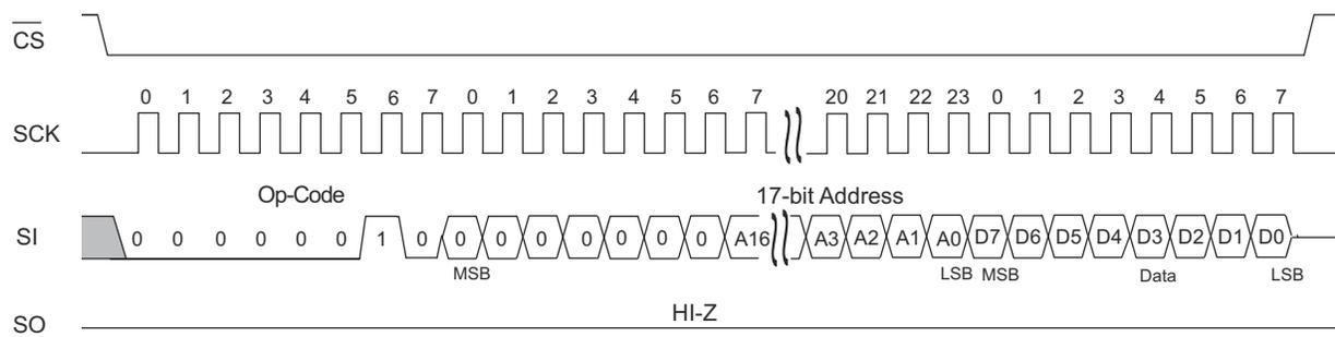
**Figure 15. Burst Mode Write Instruction Timing**
