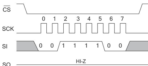
To issue this instruction, the device must be write enabled (WEN bit = '1'). The instruction is performed by transmitting the STORE opcode on the SI pin following the falling edge of CS. The WEN
