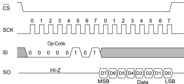
**Figure 7. Fast Read Status Register (FAST\_RDSR) Instruction Timing**
