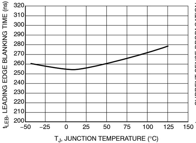
Figure 18. Leading Edge Blanking Time vs. Junction Temperature
