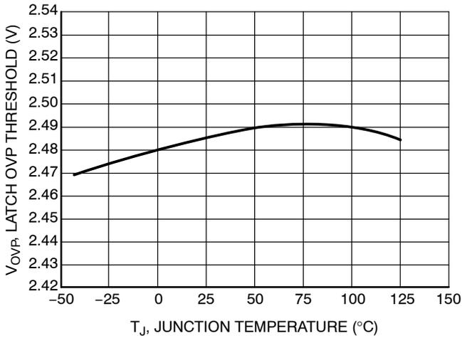
Figure 34. Latch OVP Threshold vs. Junction Temperature
