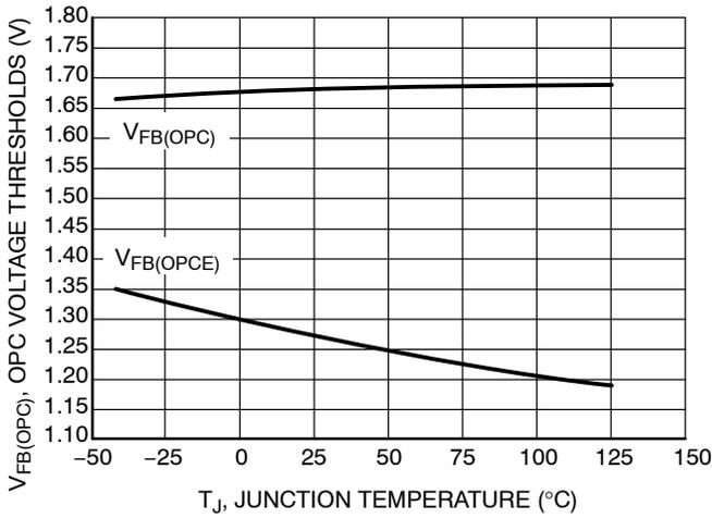
Figure 22. OPC FB Thresholds vs. Junction Temperature
