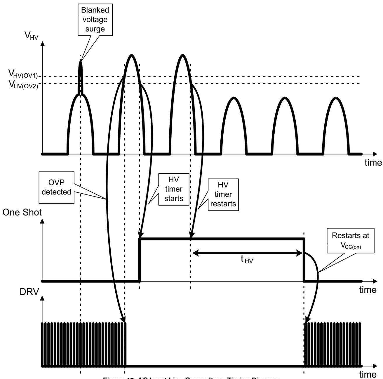
Figure 45. AC Input Line Overvoltage Timing Diagram
