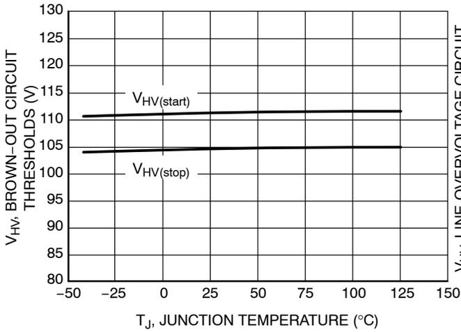
Figure 10. Brown-Out Circuit Thresholds vs. Junction Temperature
