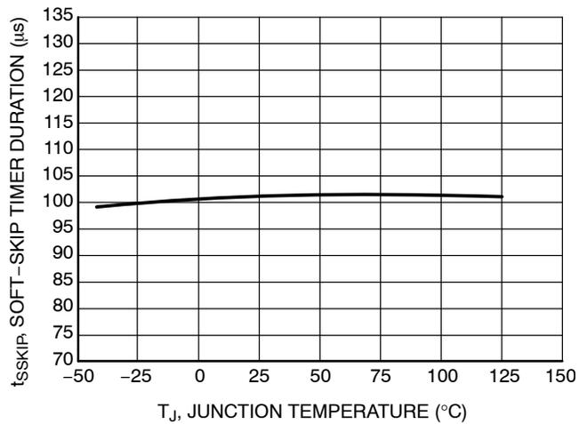
Figure 33. Soft-Skip Timer Duration vs. Junction Temperature
