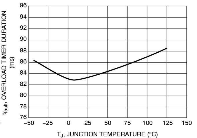
Figure 27. Overload Timer Duration vs. Junction Temperature
