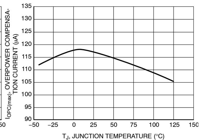
Figure 21. Overpower Compensation Current vs. Junction Temperature
