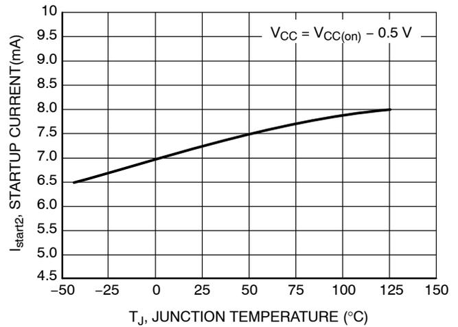
Figure 7. Startup Current vs. Junction Temperature
