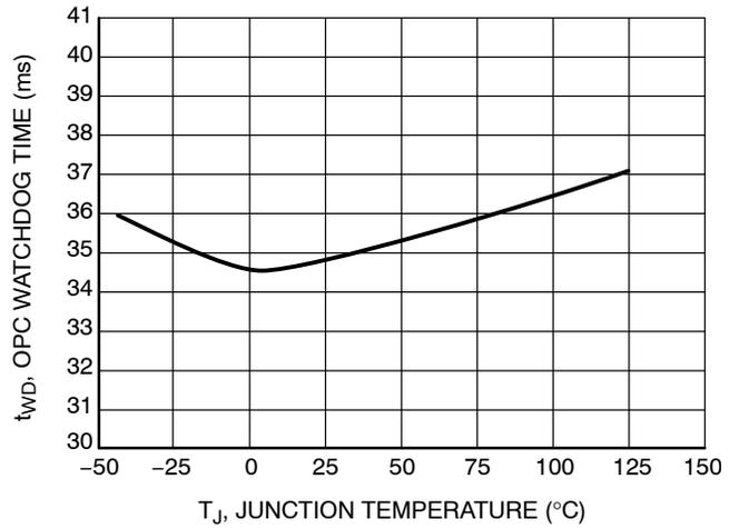
Figure 23. OPC Watchdog Time Thresholds vs. Junction Temperature
