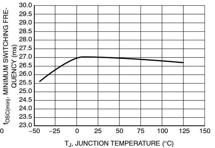
Figure 31. Minimum Switching Frequency vs. Junction Temperature
