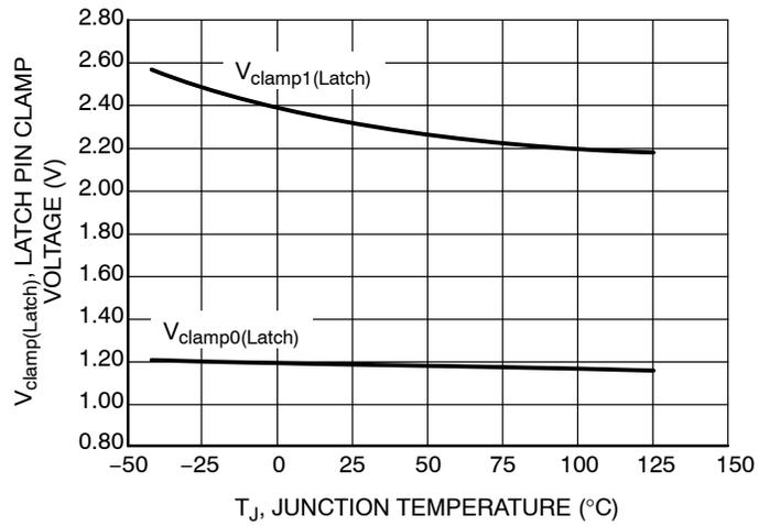
**Figure 40. Latch Pin Clamp Voltage vs. Junction Temperature**
