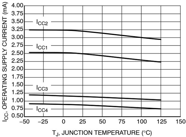
Figure 12. I<sub>CC</sub> Supply Currents vs. Junction Temperature
