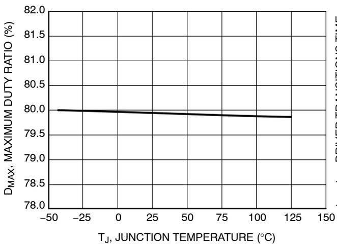
Figure 14. Maximum Duty Ratio vs. Junction Temperature
