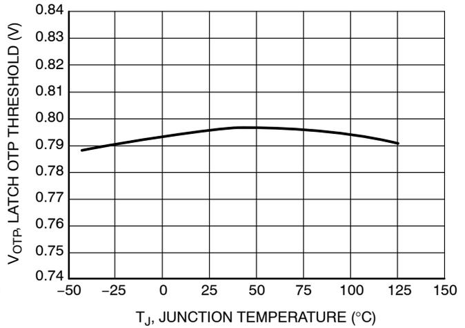
Figure 35. Latch OTP Threshold vs. Junction Temperature
