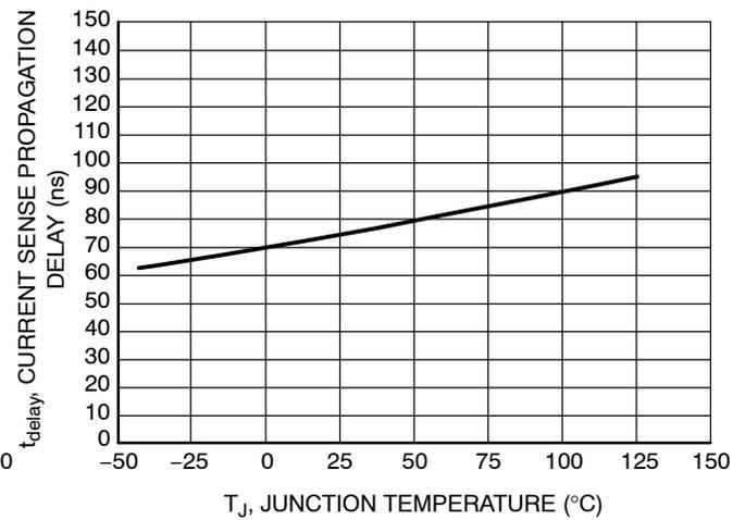
Figure 19. Current Sense Propagation Delay vs. Junction Temperature
