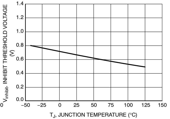
Figure 5. Inhibit Threshold Voltage vs. Junction Temperature
