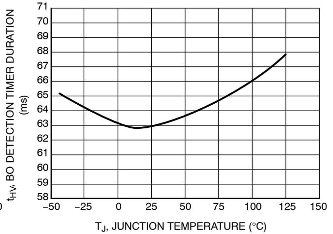
Figure 29. Brown-Out Detection Timer Duration vs. Junction Temperature
