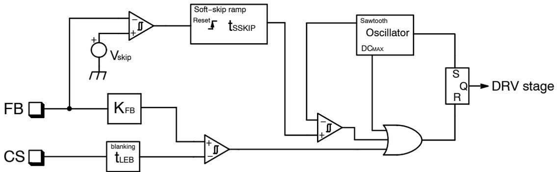
Figure 60. Skip Cycle with Soft-Skip Schematic
