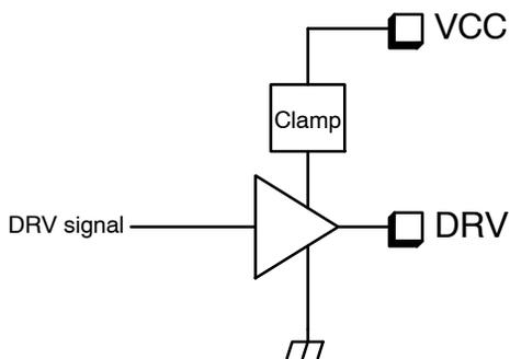
Figure 47. Clamped Driver
