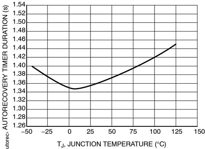
Figure 28. Autorecovery Timer Duration vs. Junction Temperature
