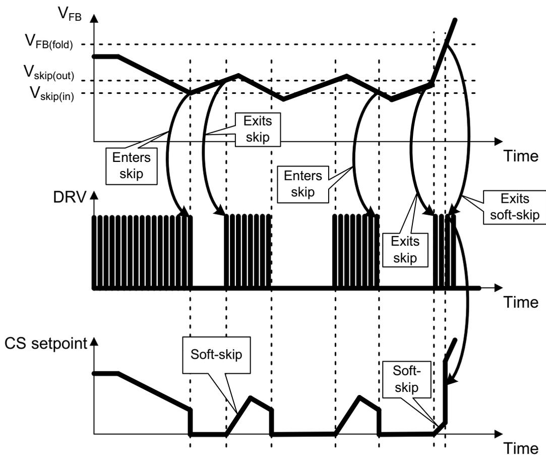
Figure 61. Skip Cycle with Soft-Skip Timing Diagram
