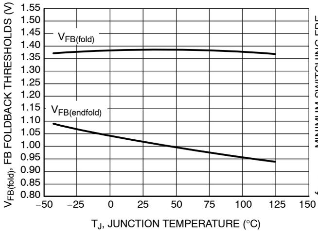
Figure 30. FB Thresholds for Frequency Foldback vs. Junction Temperature
