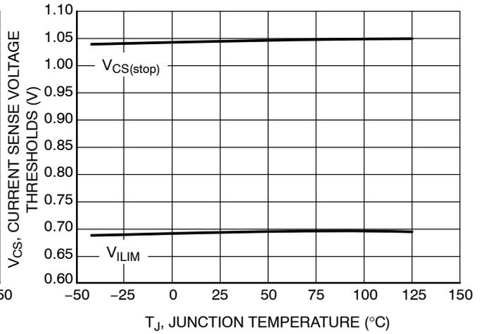
Figure 17. Current Sense Voltage Thresholds vs. Junction Temperature
