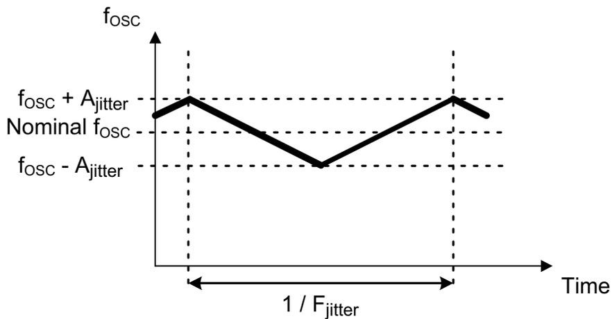
Figure 46. Frequency Jittering
