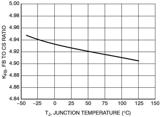
Figure 24. FB to CS Ratio vs. Junction Temperature
