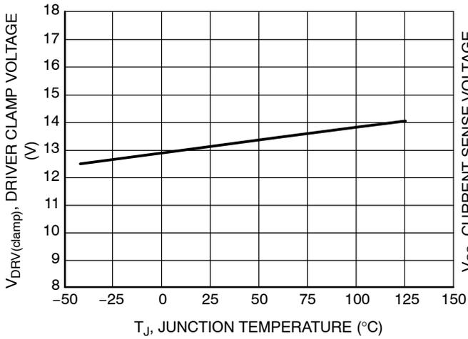
Figure 16. Driver Clamp Voltage vs. Junction Temperature
