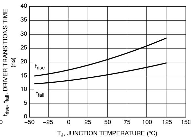
Figure 15. Driver Transitions Time vs. Junction Temperature
