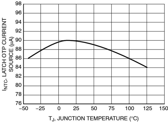
Figure 36. Latch OTP Current Source vs. Junction Temperature
