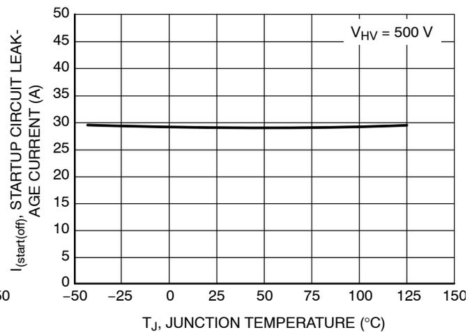
Figure 9. Startup Circuit Leakage Current vs. Junction Temperature
