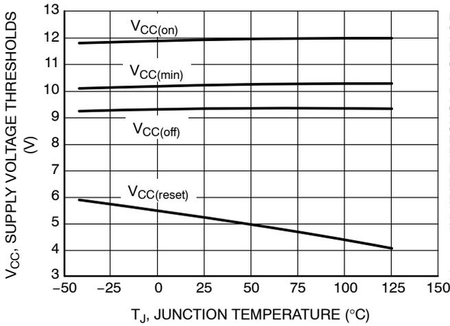
Figure 4. Supply Voltage Thresholds vs. Junction Temperature
