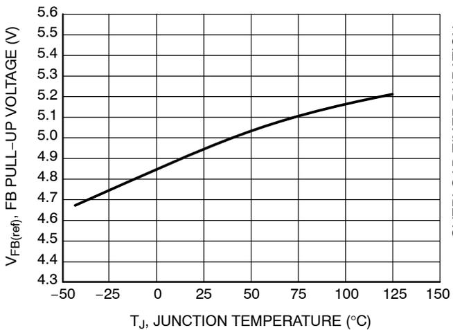
Figure 26. FB Pull-up Voltage vs. Junction Temperature
