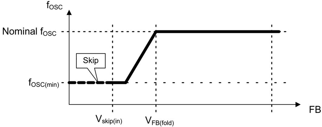
Figure 59. Frequency Foldback when the FB Voltage Decreases
