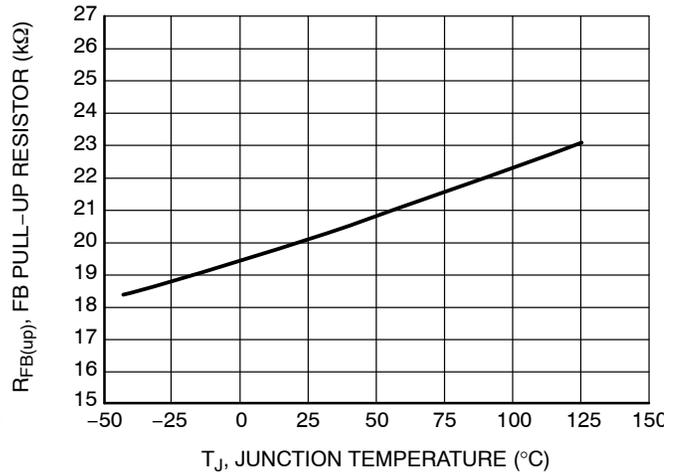
Figure 25. FB Pull-up Resistor vs. Junction Temperature
