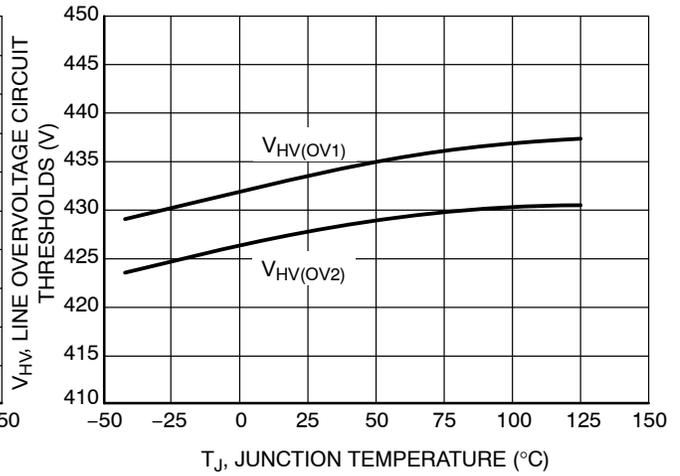
Figure 11. Line Overvoltage Circuit Thresholds vs. Junction Temperature
