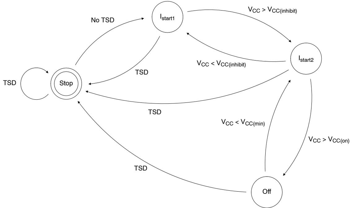
Figure 64. HV Startup Current Source State Diagram
