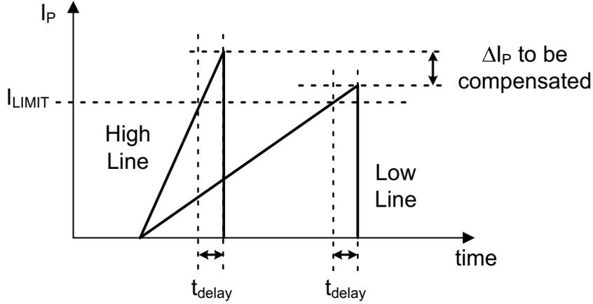
**Figure 50. Line Compensation for True Overpower Protection**
