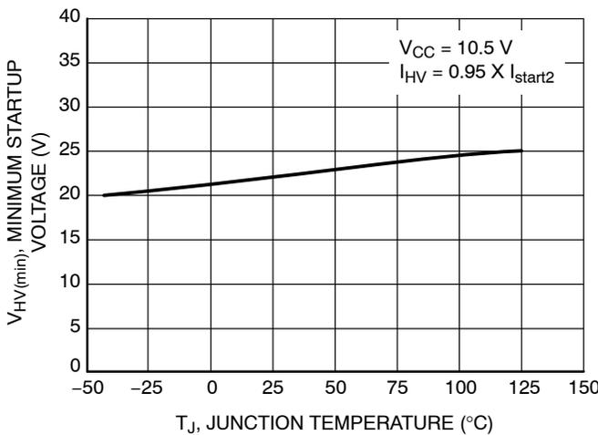
Figure 8. Minimum Startup Voltage vs. Junction Temperature
