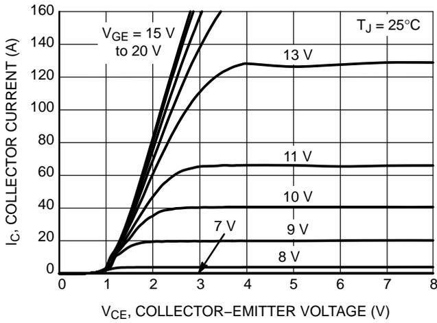
Figure 1. Output Characteristics
