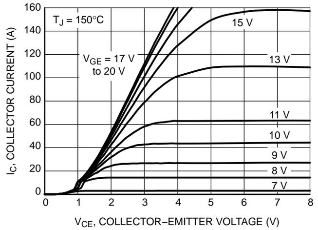
Figure 2. Output Characteristics
