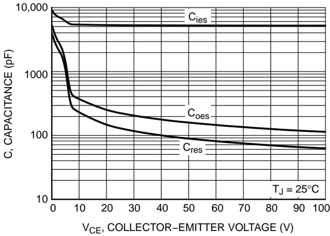
Figure 3. Typical Capacitance
