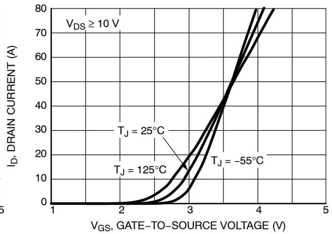
Figure 2. Transfer Characteristics
