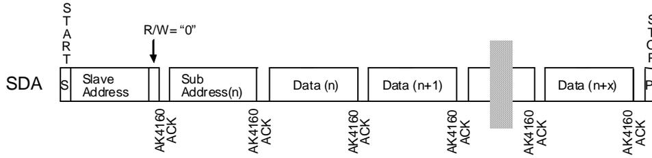
Figure 10. Data Transfer Sequence at the I<sup>2</sup>C-bus Mode
