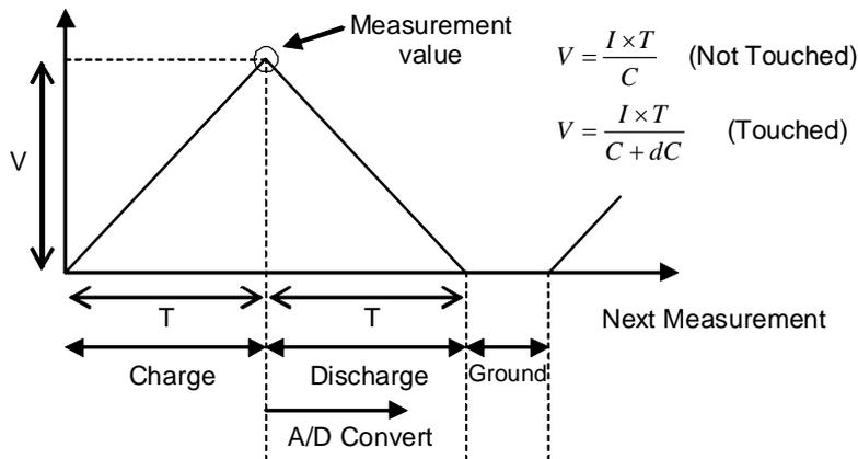
Figure 6. The Voltage Transaction of a Sense Terminal
