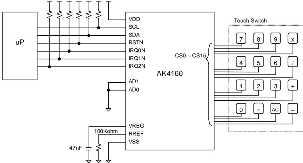
Figure 18. Typical Connection Diagram for 16ch Touch Switch
