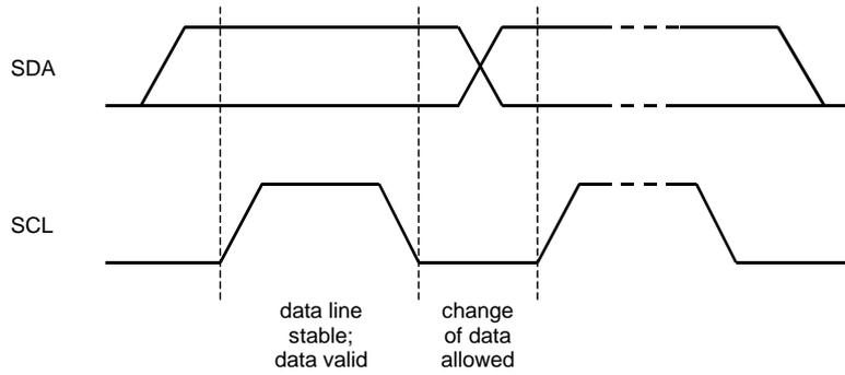
Figure 16. Bit Transfer on the I<sup>2</sup>C-Bus
