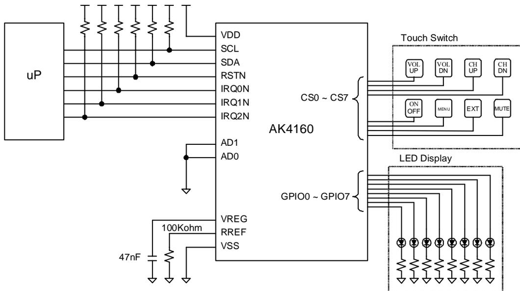
Figure 19. Typical Connection Diagram for 8ch Touch Switch & 8ch LED Display
