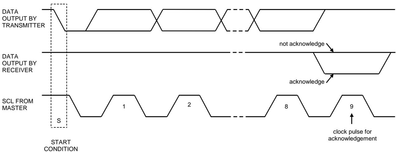
Figure 15. Acknowledge on the I<sup>2</sup>C-Bus
