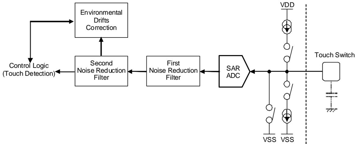
Figure 5. Touch Sensor Block Diagram
