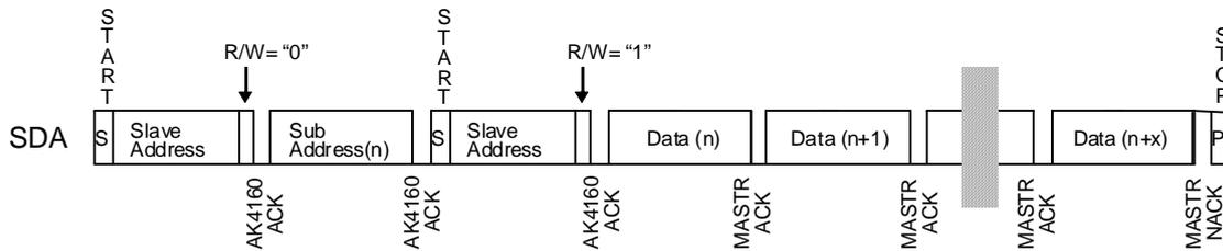
Figure 17. Register Address Read
