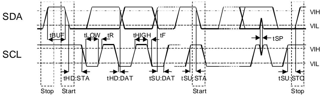
Figure 4. I<sup>2</sup>C Interface Timing Diagram
