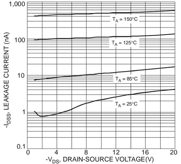
Fig. 22 Typical Drain-Source Leakage Current vs. Voltage
