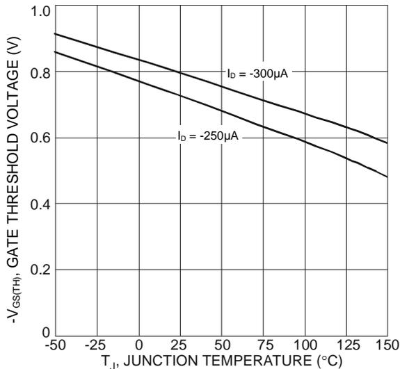
Fig. 19 Gate Threshold Variation vs. Junction Temperature
