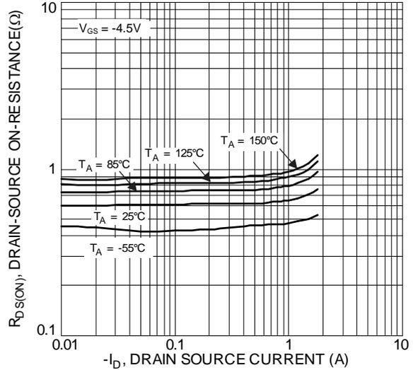
Fig. 16 Typical On-Resistance vs. Drain Current and Temperature
