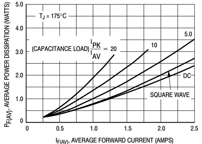
**Figure 5. Power Dissipation**
