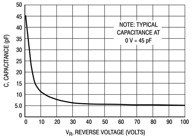
**Figure 3. Typical Capacitance**
