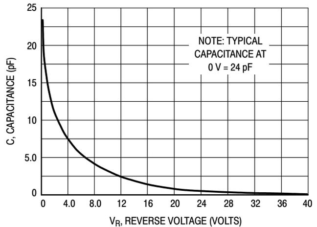
**Figure 8. Typical Capacitance**
