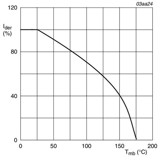
$$I_{der} = \frac{I_D}{I_{D(25^\circ\text{C})}} \times 100\%$$
