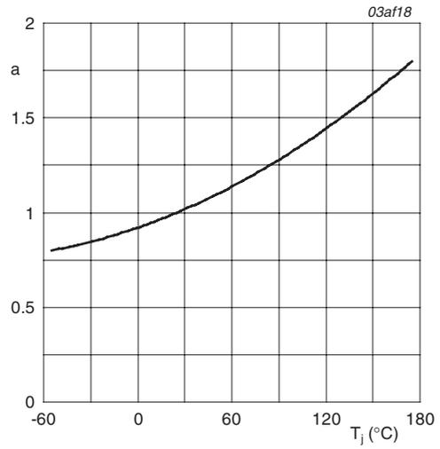
$$a = \frac{R_{DS(on)}}{R_{DS(on)(25^\circ\text{C})}}$$
