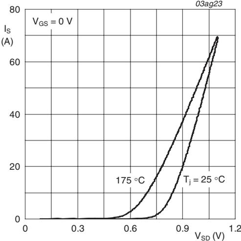
$T_j = 25\text{ °C}$  and  $175\text{ °C}; V_{GS} = 0\text{ V}$
