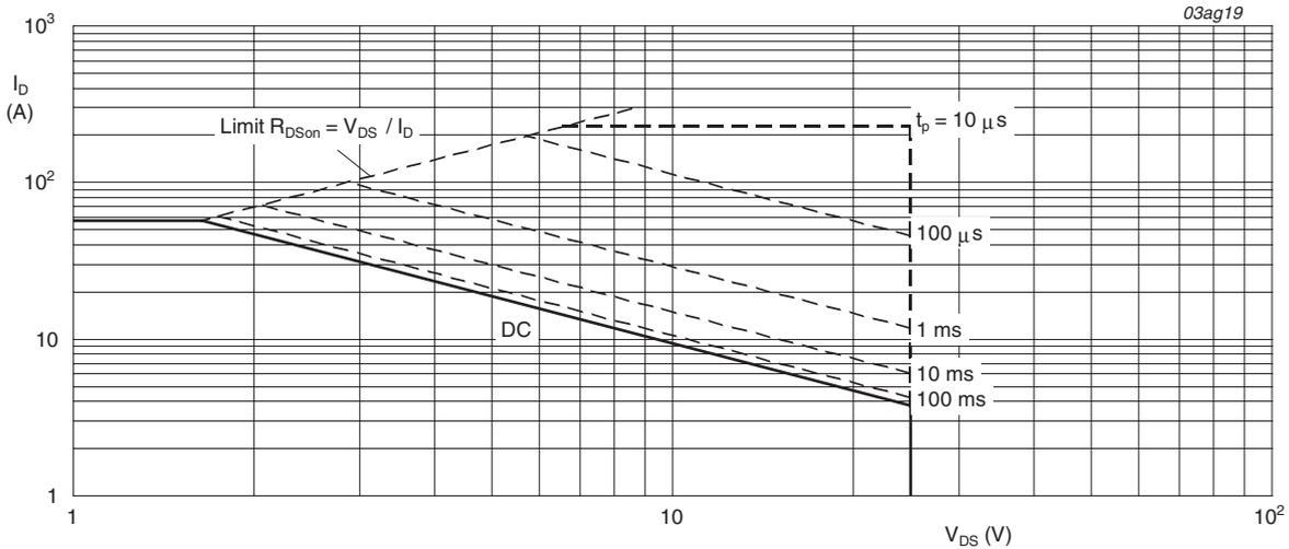
$T_{mb} = 25^\circ\text{C}; I_{DM}$  is single pulse;  $V_{GS} = 5\text{V}$
