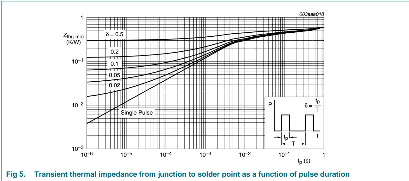
**Fig 5. Transient thermal impedance from junction to solder point as a function of pulse duration**
