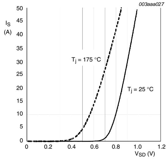
$T_j = 25^\circ C$  and  $175^\circ C; V_{GS} = 0V$
