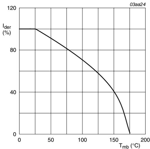
$$I_{der} = \frac{I_D}{I_{D(25^\circ\text{C})}} \times 100\%$$
