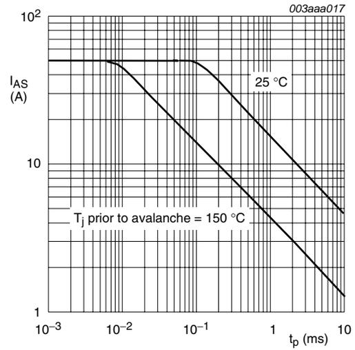
Unclamped inductive load; V<sub>DS</sub> ≤ 15V; R<sub>GS</sub> = 50Ω; V<sub>GS</sub> = 10V
