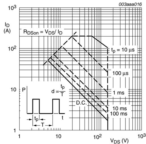
$T_{mb} = 25\text{ °C}; I_{DM}$  is single pulse
