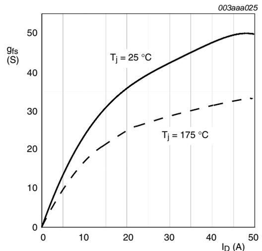
$T_j = 25^\circ\text{C}$  and  $175^\circ\text{C}; V_{DS} > I_D \times R_{DSon}$
