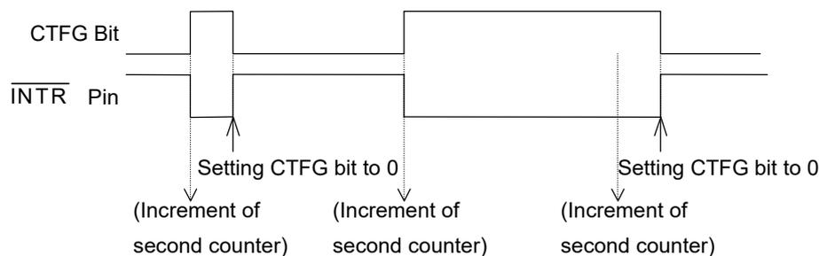
\*1), \*2) When the oscillation adjustment circuit is used, the interrupt cycle will fluctuate once per 60sec. as follows:
