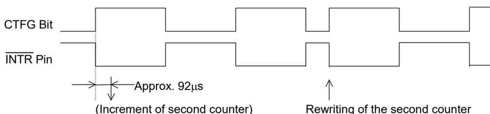
In the pulse mode, the increment of the second counter is delayed by approximately 92 µs from the falling edge of clock pulses. Consequently, time readings immediately after the falling edge of clock pulses may appear to lag behind the time counts of the real-time clocks by approximately 1 second. Rewriting the second counter will reset the other time counters of less than 1 second, driving the  $\overline{\text{INTR}}$  pin low.
