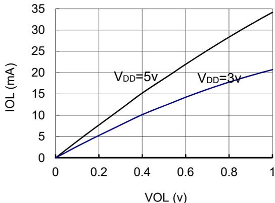
$V_{OL}$  vs.  $I_{OL}$  ( $\overline{\text{INTR}}$  pin)
