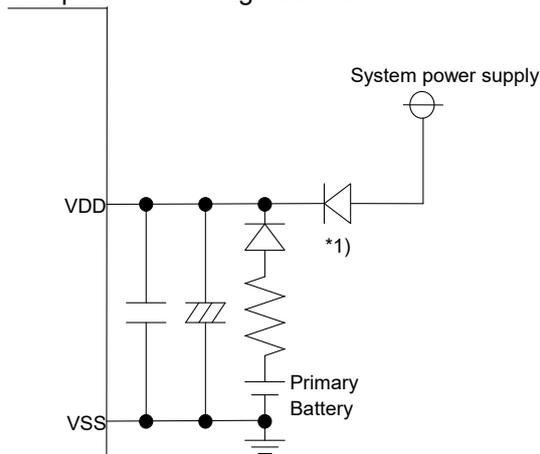
\*1) When using an OR diode as a power supply for the R2045S/D ensure that voltage exceeding the absolute maximum rating of  $V_{DD}+0.3V$  is not applied to the SO pin.
