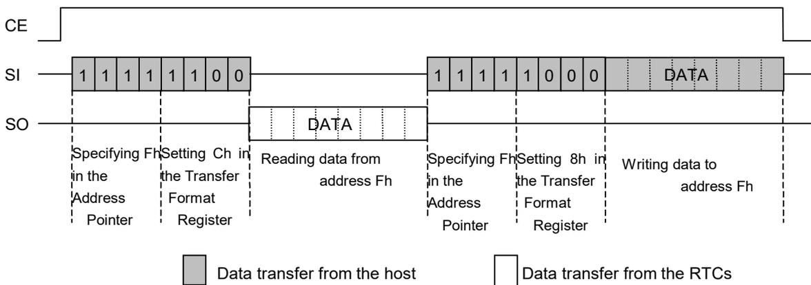
The reading and writing data transfer formats correspond to the settings in the transfer format register as shown in the table below.
