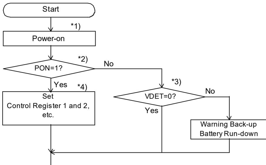
\*1) After power-on from 0 volt, the start of oscillation and the process of internal initialization require a time span on the order of 1 to 2sec, so that access should be done after the lapse of this time span or more.
