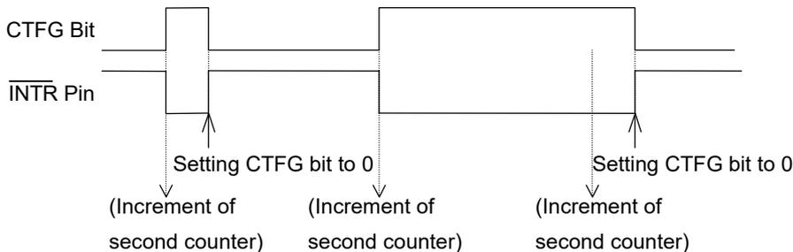
\*1), \*2) When the oscillation adjustment circuit is used, the interrupt cycle will fluctuate once per 20sec. as follows:
