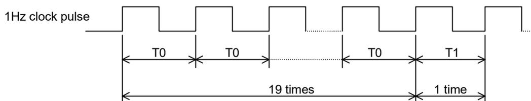
Measure the interval of T0 and T1 with frequency counter. A frequency counter with 7 or more digits is recommended for the measurement.
