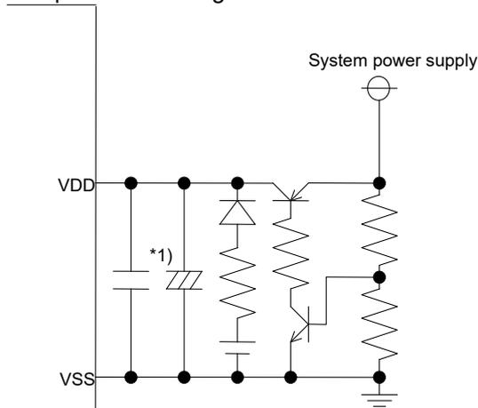
\*1) Install bypass capacitors for high frequency and low frequency applications in parallel in close vicinity to the R2045S/D.
