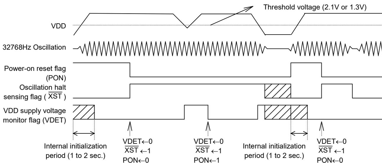
When the PON bit is set to 1 in the control register 2, the DEV, F6 to F0, WALE, DALE,  $\overline{12}/24$ ,  $\overline{CLEN2}$ , TEST, CT2, CT1, CT0, VDLS, VDET,  $\overline{CLEN1}$ , CTFG, WAFG, and DAFG bits are reset to 0 in the oscillation adjustment register, the control register 1, and the control register 2. The PON bit is also set to 1 at power-on from 0 volts.
