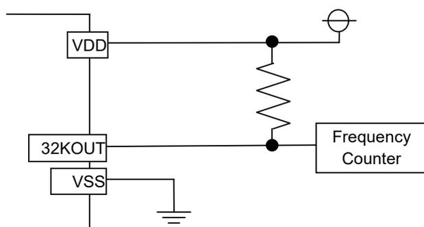
\* 1) When power-on, the R2045S/D is configured to generate 32.768-kHz clock pulses for output from the 32KOUT pin.
