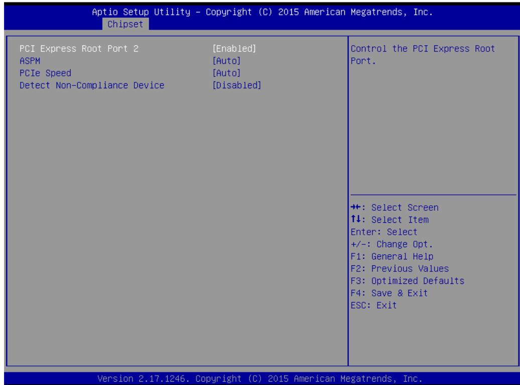
**Figure 3.31 PCI Express Root Port 2 Configuration**
