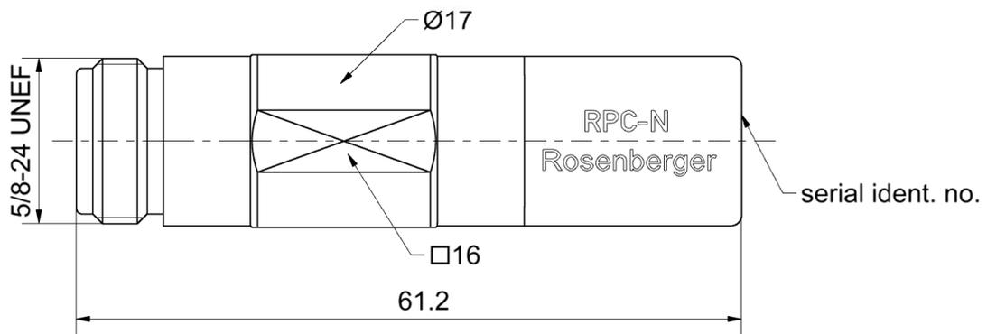
All dimensions are in mm; tolerances according to ISO 2768 m-H
