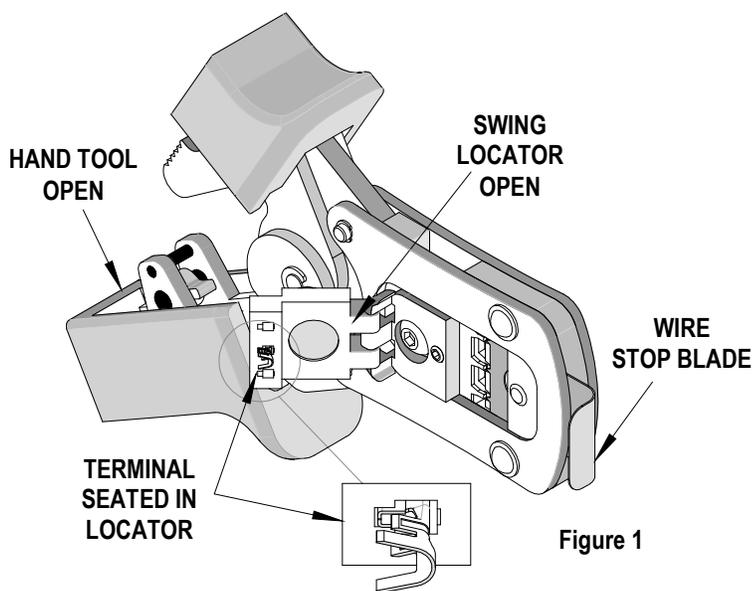
2. Insert the terminal into the correct profile until the terminal is fully seated and stops. Make sure the wire stop blade is fully seated on the terminal behind the conductor grip section.
