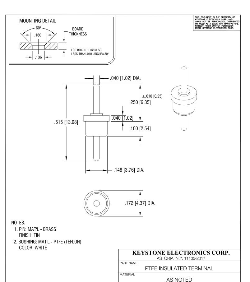
DRN BY FINISH DATE 11.28.07 N.T. **AS NOTED** APP'D SCALE LN 5X TOLERANCES INCH [MM] CODE DWG NO.  $\pm .005 [\pm 0.15]$ DECIMAL 11155 С ANGULAR ± 1° REV. DATE **DESCRIPTION** UNLESS OTHERWISE SPECIFIED
