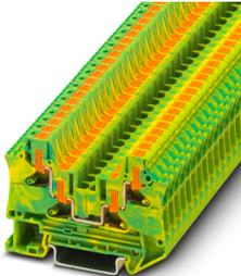
Ground modular terminal block, number of connections: 2, number of positions: 1, connection method: Push-in connection, Rated cross section: 6 mm<sup>2</sup>, cross section: 0.5 mm<sup>2</sup> - 10 mm<sup>2</sup>, mounting type: NS 35/7,5, NS 35/15, color: green/yellow
