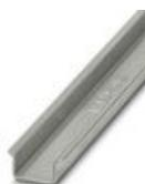
DIN rail, unperforated, acc. to EN 60715, material: Steel, galvanized, passivated with a thick layer, Standard profile 2.3 mm, color: silver
