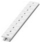
Zack marker strip, Strip, white, labeled, can be labeled with: CMS-P1-PLOTTER, Printed vertically: consecutive numbers 1 ... 10, 11 ... 20, etc. up to 91 ... 100, mounting type: snap into tall marker groove, for terminal block width: 8.2 mm, lettering field size: 10.5 x 8.15 mm, Number of individual labels: 10
