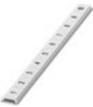
Zack Marker strip, flat, Strip, white, labeled, printed horizontally: consecutive numbers 1 ... 10, 11 ... 20, etc. up to 101 ... 110, mounting type: snap into flat marker groove, for terminal block width: 8 mm, lettering field size: 5.15 x 8.15 mm, Number of individual labels: 10
