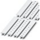
Marker for terminal blocks. Strip, white, labeled, can be labeled with: CMS-P1-PLOTTER, horizontal: L1, L2, L3, N, PE, L1, L2, L3, N, PE, mounting type: snap into tall marker groove, for terminal block width: 8.2 mm, lettering field size: 10.5 x 8.15 mm, Number of individual labels: 10
