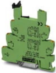
6.2 mm PLC basic terminal block for output functions with push-in connection, without relay or solid-state relay, for mounting on DIN rail NS 35/7,5, with load return line connection (BB), 1 N/O contact, input voltage 24 V DC
