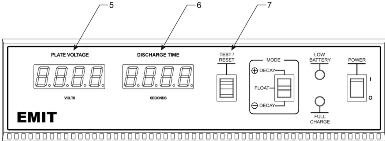
Figure 3-2: Front Panel Features (cont.)
