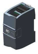
SIPLUS S7-1200 SM 1221 16DI, based on 6ES7221-1BH32-0XB0 with conformal coating, -20...+60  $^{\circ}\text{C},$  16 DI, 24 V DC, sink/source
