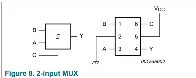
Figure 8. 2-input MUX
